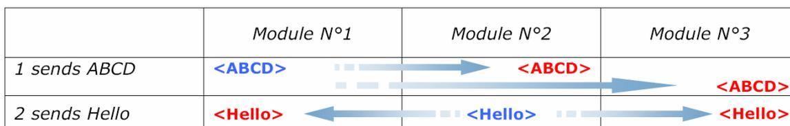
In this mode the RF modem appears as a wireless serial point-to-point link, reproducing the function of a half duplex serial cable<sup>8</sup>.
