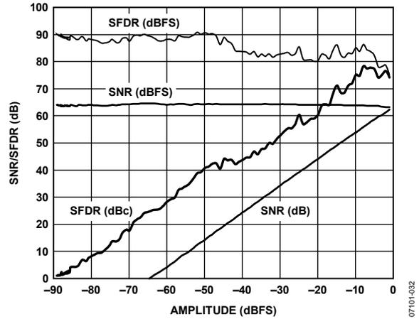
Figure 10. SNR/SFDR vs. Input Amplitude; 140.3 MHz
