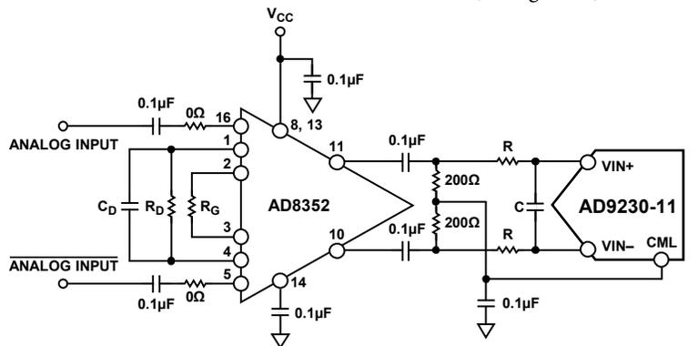
Figure 23. Differential Input Configuration Using the AD8352
