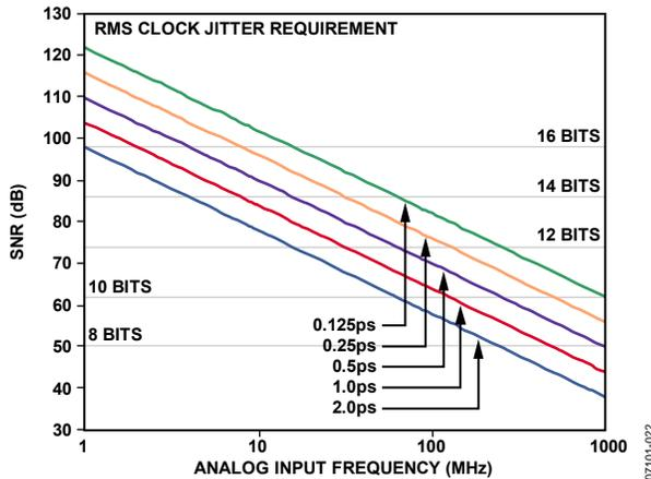
Figure 29. Ideal SNR vs. Input Frequency and Jitter
