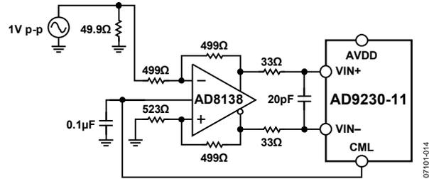
Figure 21. Differential Input Configuration Using the AD8138
