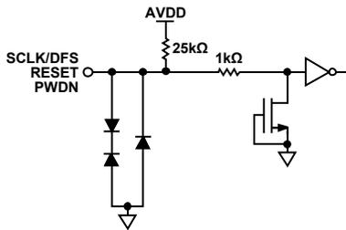
Figure 17. Equivalent SCLK/DFS, RESET, PWDN Input Circuit
