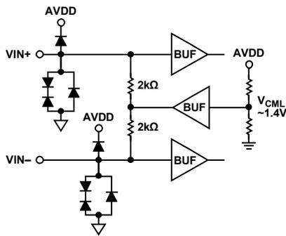
Figure 16. Analog Inputs ( $V_{CM} = \sim 1.4V$ )
