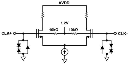
Figure 15. Clock Inputs
