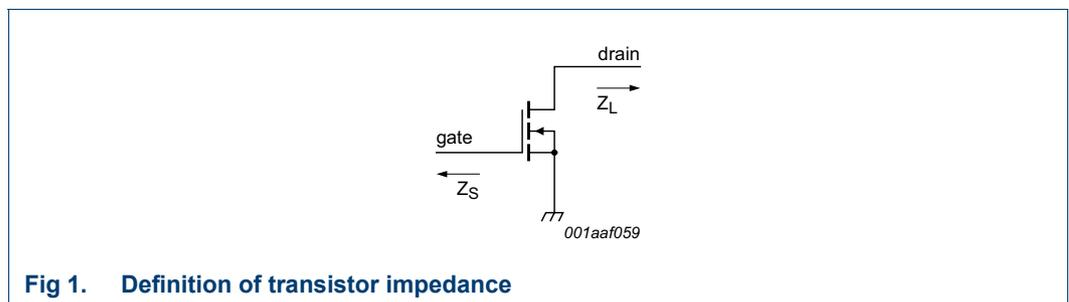
**Fig 1. Definition of transistor impedance**
