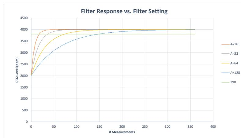
The graph above shows the effect of the filter on response times. Increasing the filter setting increases the measurement output response time. T<sub>90</sub> is the time to 90% of reading. The CozIR®-LP takes 2 readings per second. The CozIR®-LP sensor will also output the raw unfiltered CO<sub>2</sub> measurement data. This data can be post processed using alternative filter algorithms.
