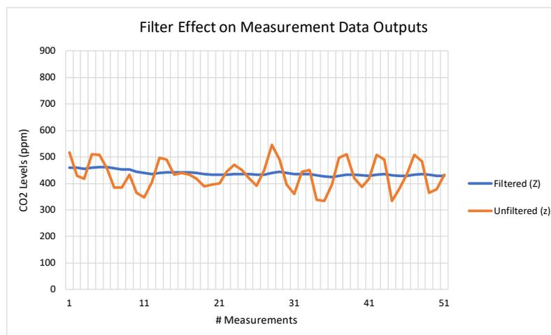
The graph above shows the effects of the filter on the CO<sub>2</sub> measurement data (Z). The unfiltered output (z) is shown in orange and the filtered output (Z) shown in blue.
