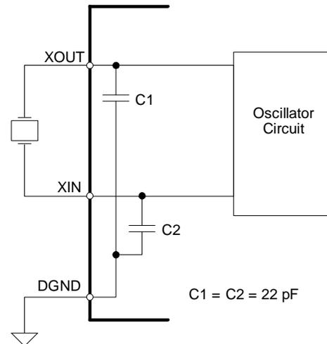
**Figure 3. Oscillator Connection**
