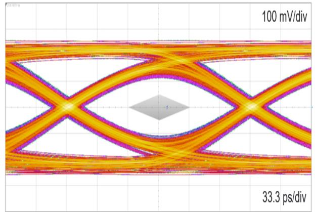
**Figure 12. MIPI D-PHY 2.5 Gbps long reference channel eye diagram without ECMF04-4HSWM10**
