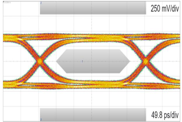
**Figure 10. USB3.2 Gen 1 5.0 Gbps eye diagram without ECMF04-4HSWM10 (with worst cable and equalizer)**
