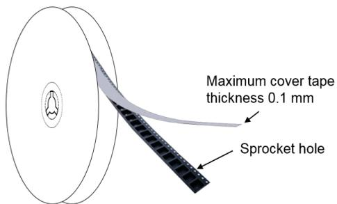
Figure 24. Reel dimensions (mm)
