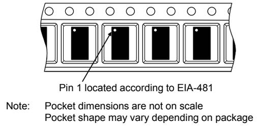
Figure 23. Tape and reel orientation
