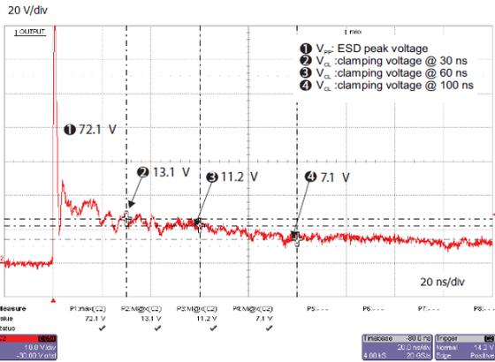
**Figure 5. ESD response to IEC61000-4-2 (-8 kV contact discharge)**
