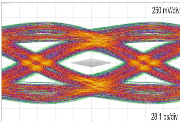
**Figure 7. HDMI2.0 - 5.94 Gbps eye diagram with device**
