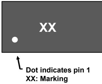
Figure 22. Package orientation in reel
