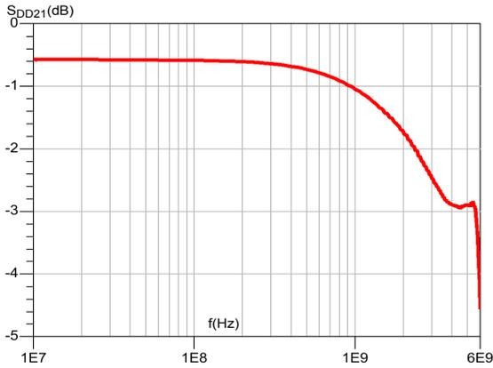
**Figure 3. Common mode attenuation versus frequency**
