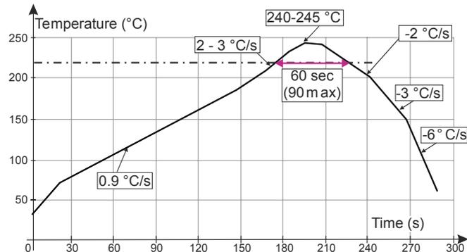
**Note:** Minimize air convection currents in the reflow oven to avoid component movement. Maximum soldering profile corresponds to the latest IPC/JEDEC J-STD-020.
