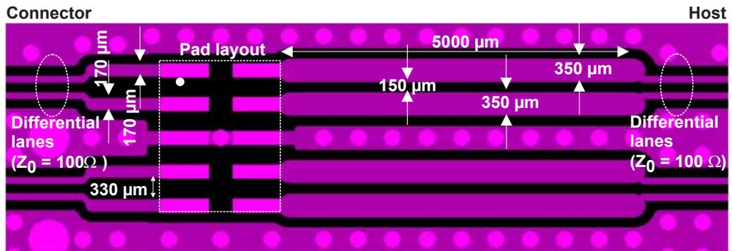
Figure 20. PCB stack dimensions
