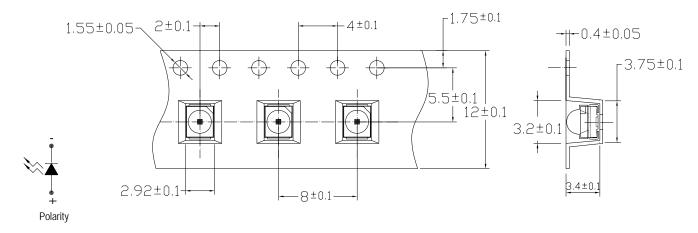
**Note:** The tolerances unless mentioned is  $\pm 0.1$ mm Unit = mm
