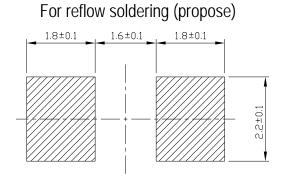
**Note:** Tolerances Unless Dimension  $\pm 0.1$ mm, Unit = mm
