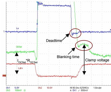
Fig. 9: OCset pin during normal condition
