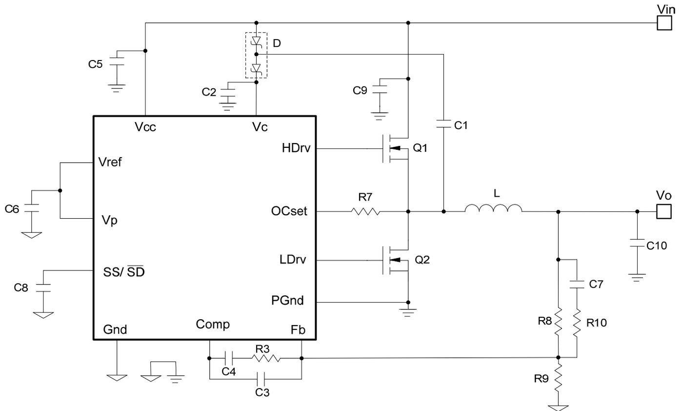
Fig.16: Application circuit for 12V to 0.9V
