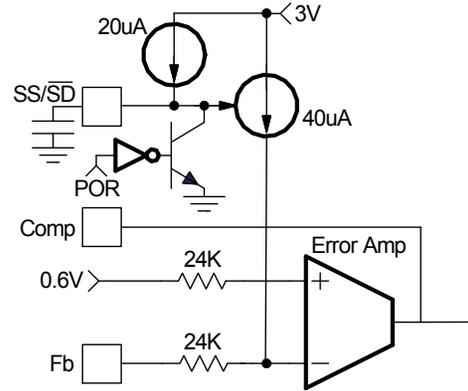
Fig. 5: Soft-Start circuit for IR3628
