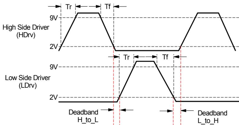
Fig. 3: Definition of Rise/Fall time and Deadband Time
