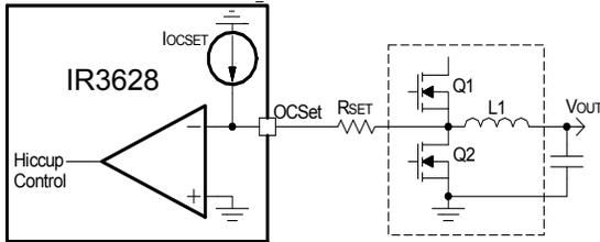
Fig. 7: Connection of over current sensing resistor
