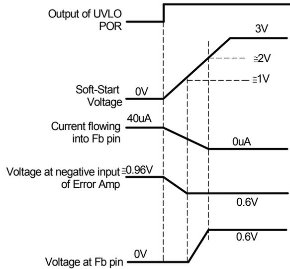
Fig. 6: Theoretical operation waveforms during soft-start
