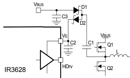
Fig. 11: Charge pump circuit to generate Vc voltage
