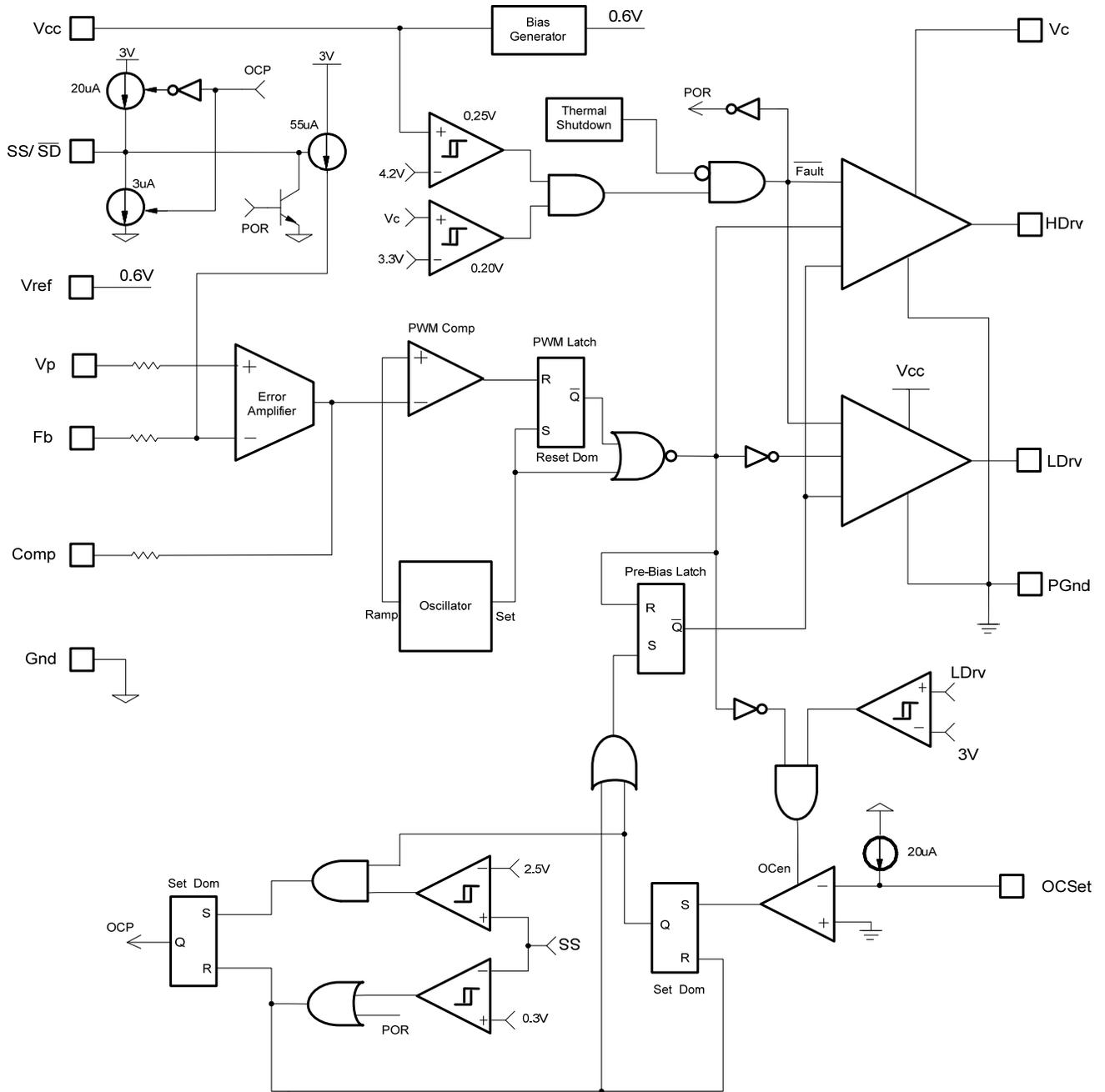
Fig. 2: Simplified block diagram of the IR3628
