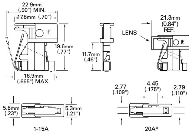
\*20A Fuseholder must be used. Fuse is keyed to prevent insertion in lower rated holders. 20A Fuseholder is designed to accept all ratings up to 20 amperes.
