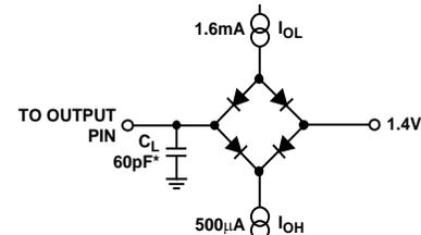
\*IN SERIAL INTERFACE MODES, THE SYNC, SCLK, AND SDOUT TIMINGS ARE DEFINED WITH A MAXIMUM LOAD  $C_L$  OF 10pF; OTHERWISE, THE LOAD IS 60pF MAXIMUM.
