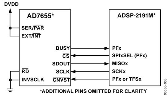
Figure 34. Interfacing the AD7655 to SPI Interface
