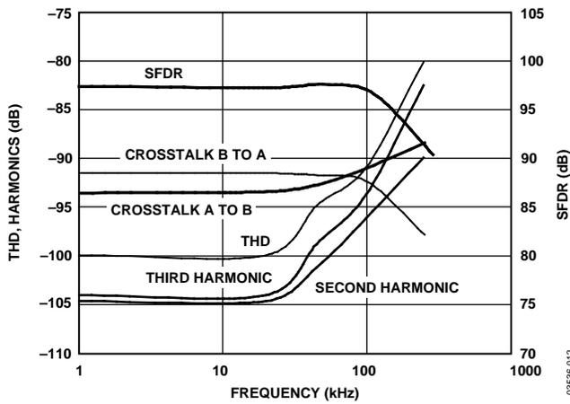
Figure 13. THD, Harmonics, Crosstalk, and SFDR vs. Frequency
