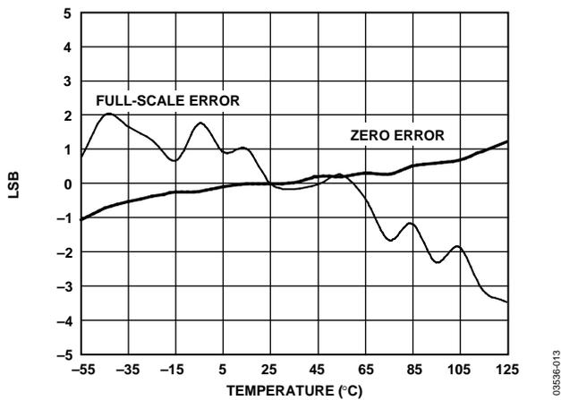
Figure 14. Full-Scale Error and Zero Error vs. Temperature
