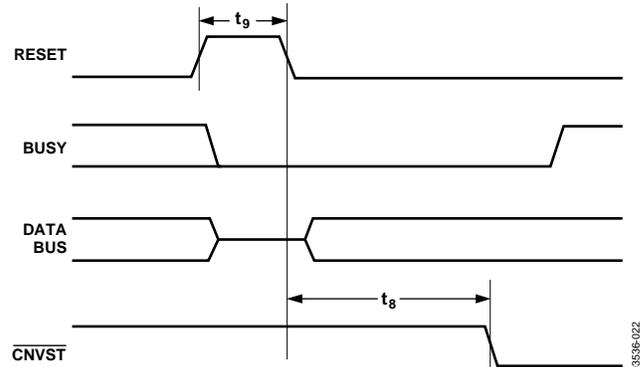
Figure 23. Reset Timing
