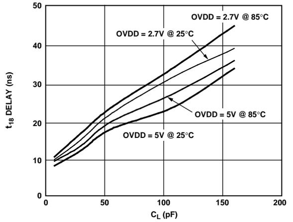
Figure 16. Typical Delay vs. Load Capacitance  $C_L$
