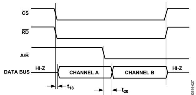
Figure 28. A/ $\overline{B}$  Channel Reading
