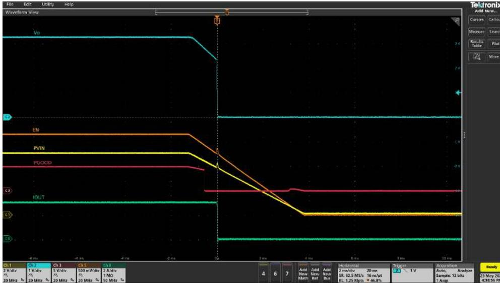
Figure 15 Shutdown with VCC UVLO at 3A load (Ch1: P<sub>VIN</sub>, Ch2: V<sub>OUT</sub>, Ch3: PG, Ch5: Enable, Ch8: I<sub>OUT</sub>)
