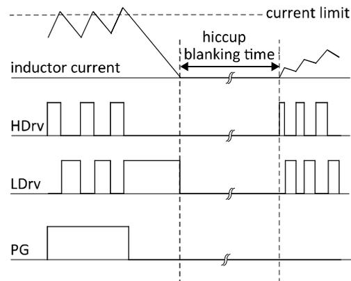
**Figure 9 Illustration of OCP in hiccup mode**
