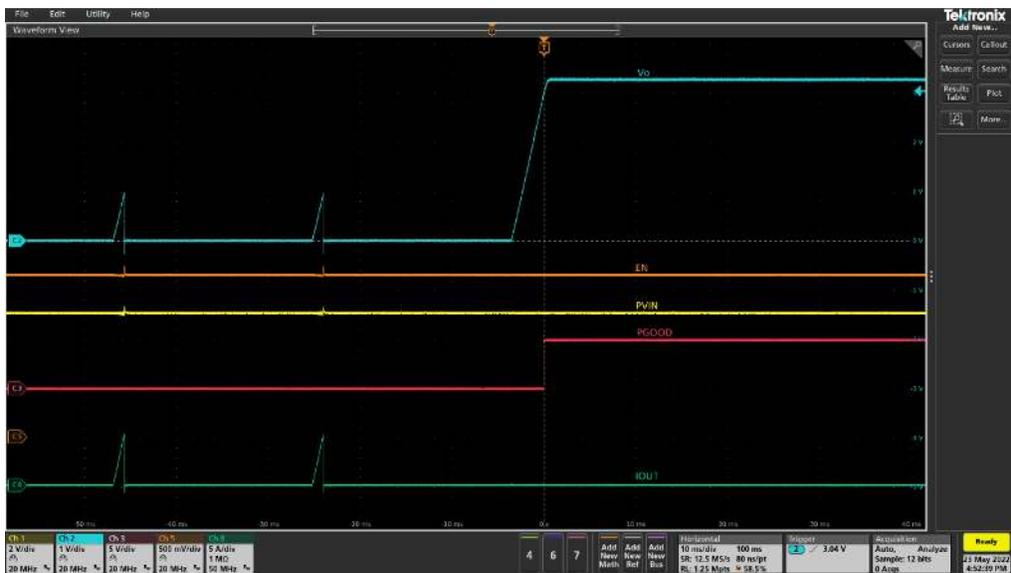
**Figure 18 Over-current protection and auto-recover to 3A (Ch1:  $V_{IN}$ , Ch2:  $V_{OUT}$ , Ch3: PG, Ch5: Enable, Ch8:  $I_{OUT}$ )**
