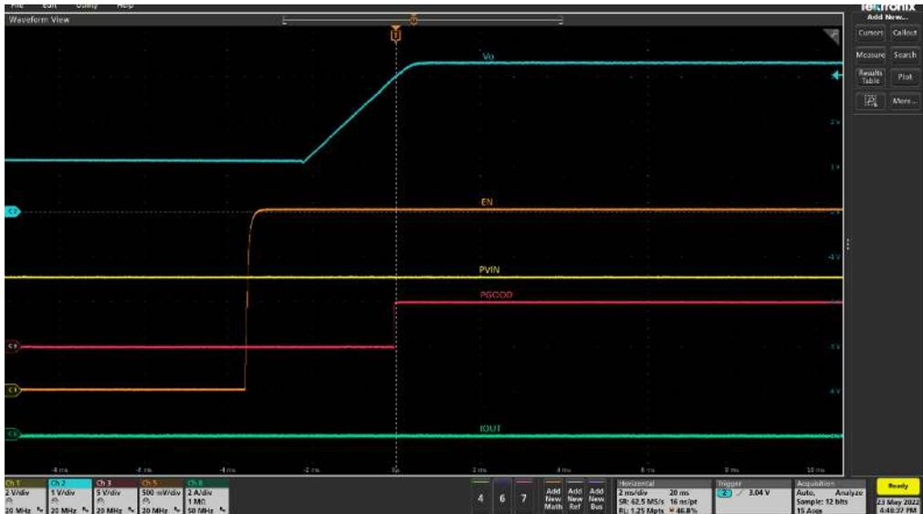
**Figure 17 Startup into pre-bias (Ch1:  $V_{IN}$ , Ch2:  $V_{OUT}$ , Ch3: PG, Ch5: Enable, Ch8:  $I_{OUT}$ )**
