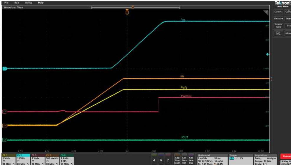
**Figure 13 Startup with no load (Ch1:PV<sub>IN</sub>, Ch2: V<sub>OUT</sub>, Ch3: PG, Ch5: Enable, Ch8:I<sub>OUT</sub>)**
