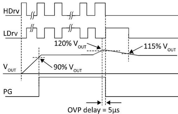
**Figure 10** Illustration of latched OVP
