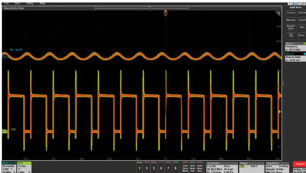
Figure 20 Sw and V<sub>OUT</sub> ripple at 3A (Ch2: V<sub>OUT</sub> Ripple, Ch4: Sw)
