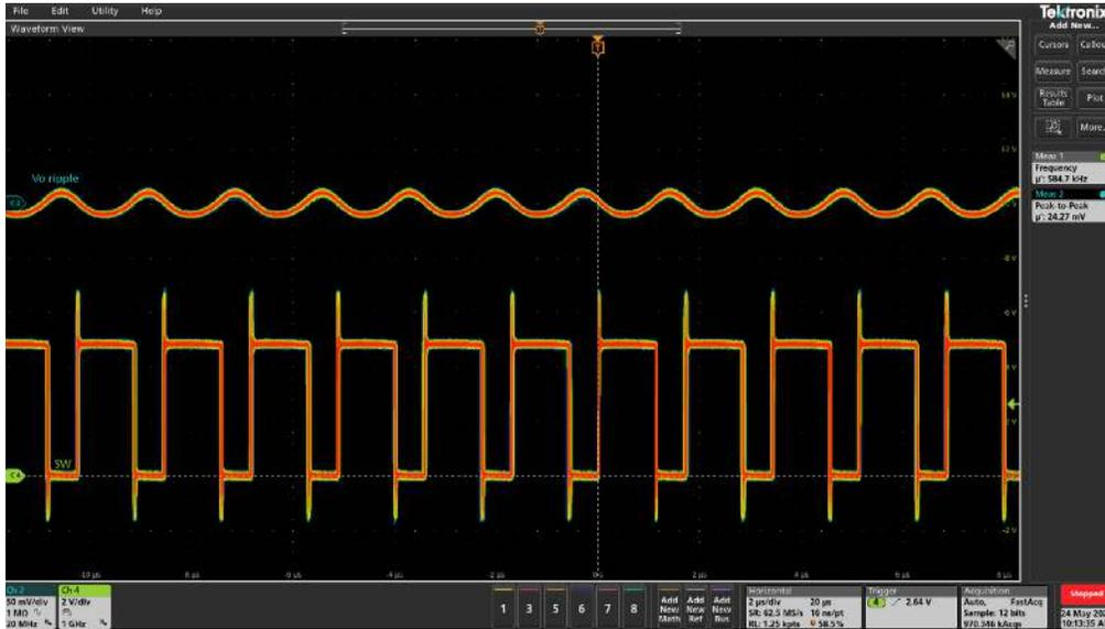
Figure 19 Sw and V<sub>OUT</sub> ripple at 0A (Ch2: V<sub>OUT</sub> Ripple, Ch4: Sw)
