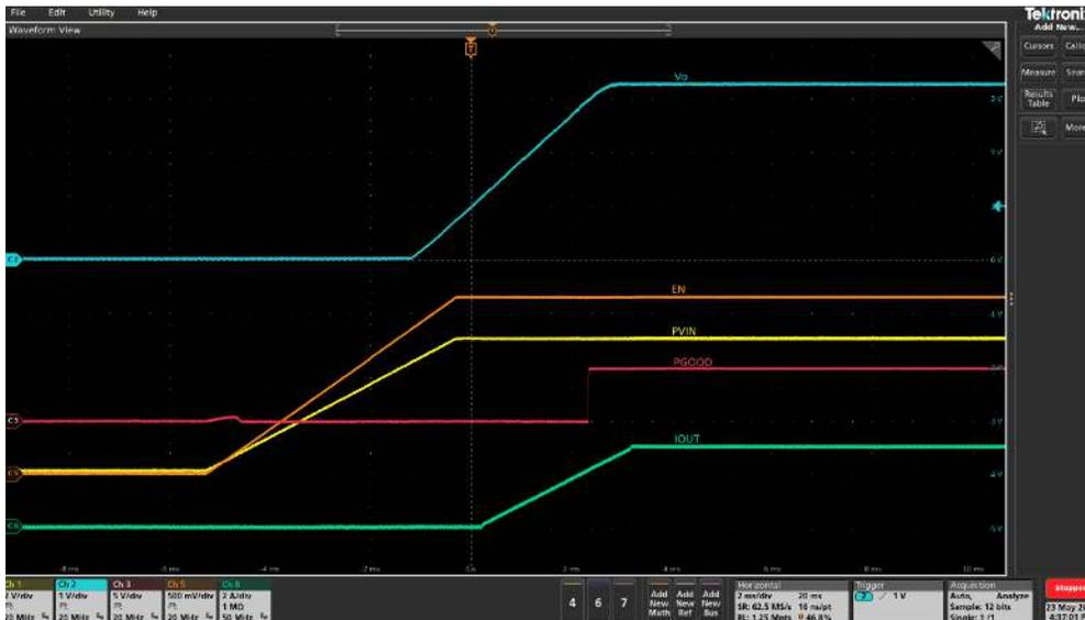
**Figure 14 Startup with 3A load (Ch1:PV<sub>IN</sub>, Ch2: V<sub>OUT</sub>, Ch3: PG, Ch5: Enable, Ch8: I<sub>OUT</sub>)**
