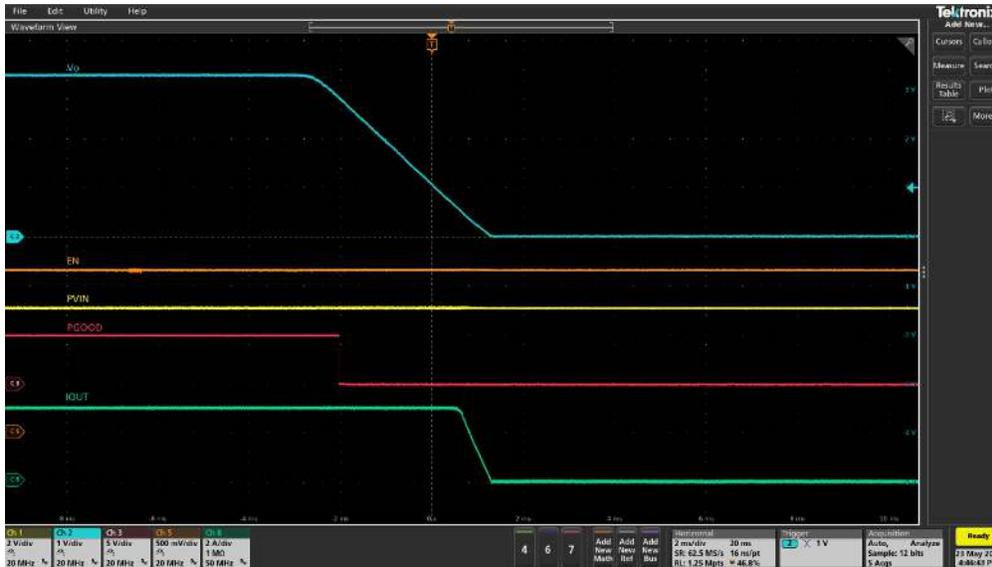
Figure 16 Soft turn off at 3A load (Ch1: P<sub>VIN</sub>, Ch2: V<sub>OUT</sub>, Ch3: PG, Ch5: Enable, Ch8: I<sub>OUT</sub>)
