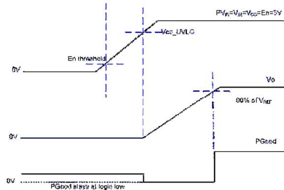
**Figure 6** Theoretical operational waveforms during soft-start
