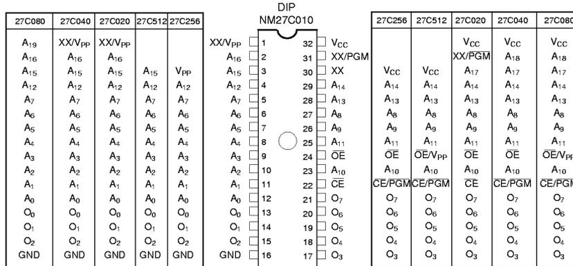
**Note:** Compatible EPROM pin configurations are shown in the blocks adjacent to the NM27C010 pins.
