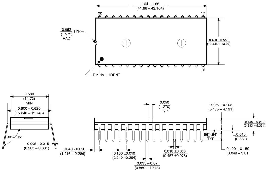
**32-Lead Molded Dual-In-Line Package (N)**
