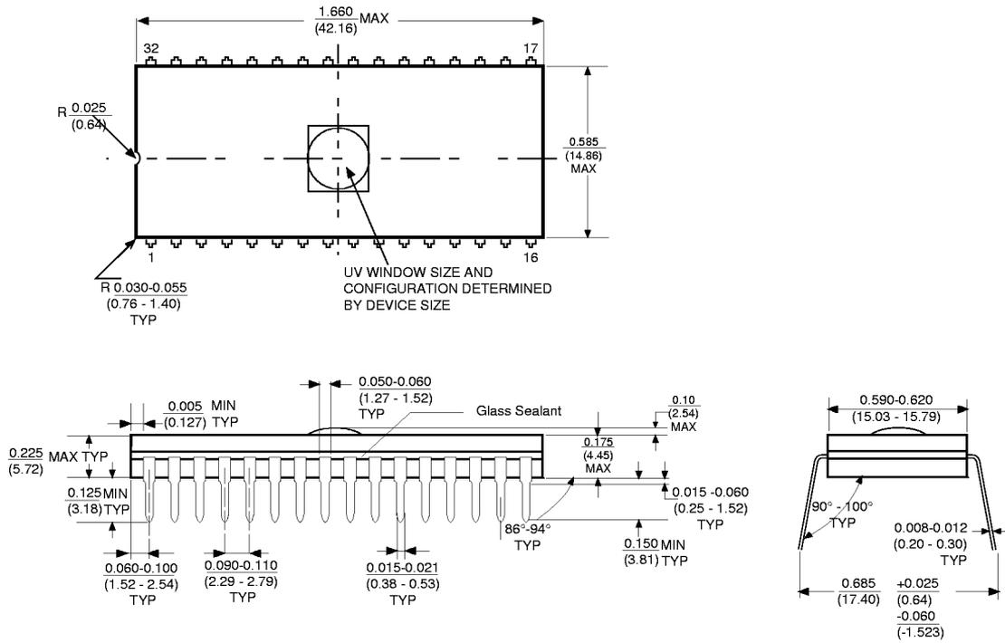
**32-Lead EPROM Ceramic Dual-In-Line Package (Q)**
