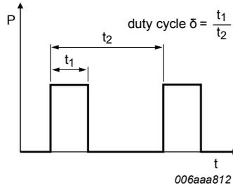
Fig. 17. Duty cycle definition
