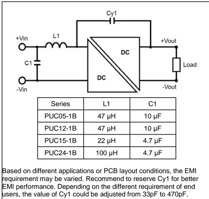
Based on different applications or PCB layout conditions, the EMI requirement may be varied. Recommend to reserve Cy1 for better EMI performance. Depending on the different requirement of end users, the value of Cy1 could be adjusted from 33pF to 470pF.
