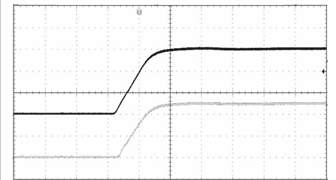
Start-up, enabled by connecting  $V_I$  at:
