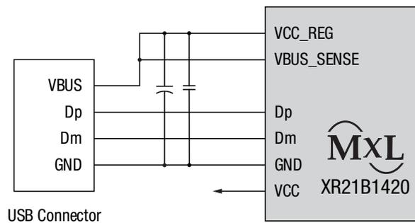
**Figure 1: Bus-Powered Mode**
