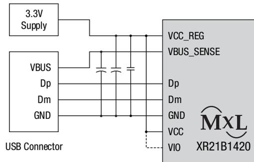
Figure 3: Self-Powered 3.3V Mode
