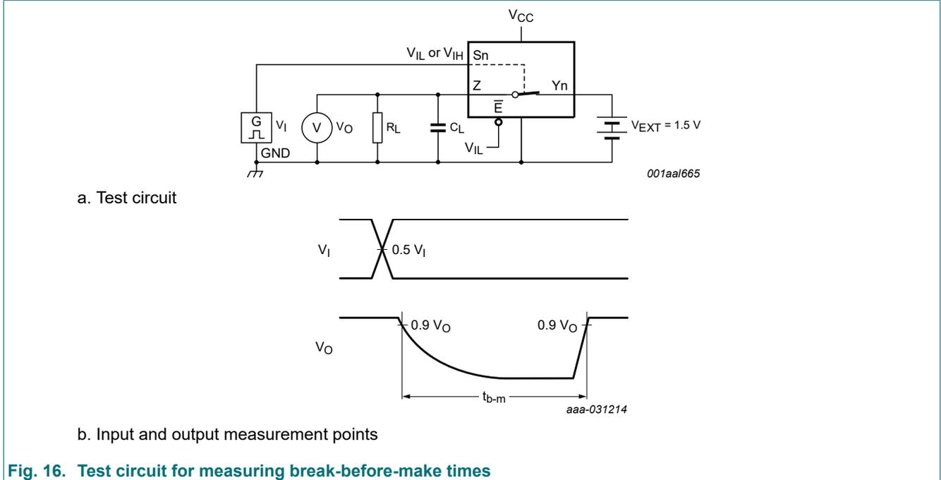
Fig. 16. Test circuit for measuring break-before-make times
