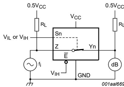
Adjust  $f_i$  voltage to obtain 0 dBm level at input.
