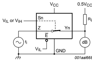
Adjust  $f_i$  voltage to obtain 0 dBm level at output. Increase  $f_i$  frequency until dB meter reads -3 dB.
