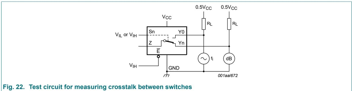
Fig. 22. Test circuit for measuring crosstalk between switches
