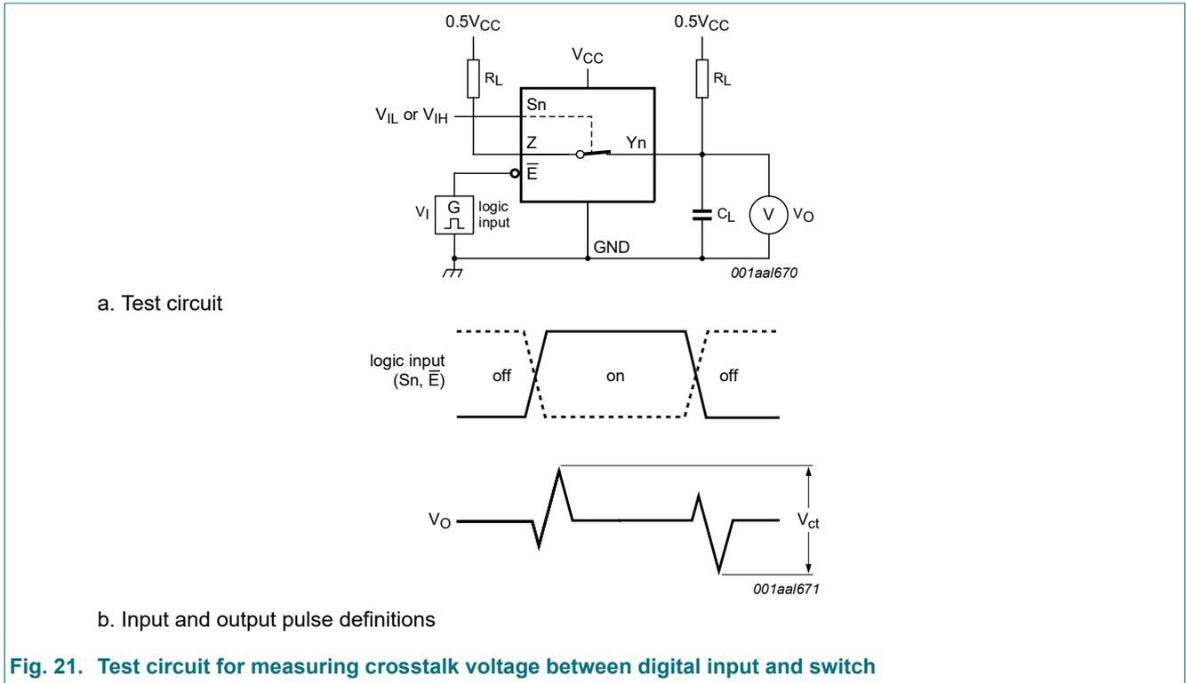
Fig. 21. Test circuit for measuring crosstalk voltage between digital input and switch
