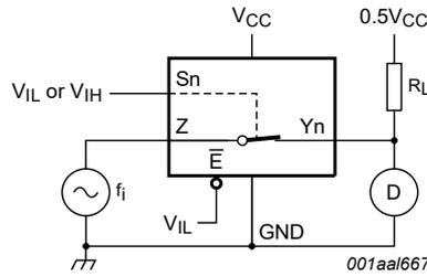
Fig. 18. Test circuit for measuring total harmonic distortion
