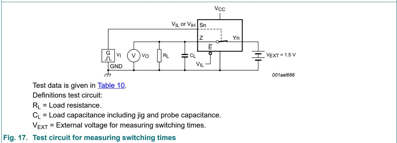
Fig. 17. Test circuit for measuring switching times
