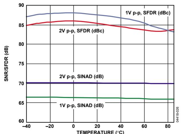
Figure 26. SINAD/SFDR vs. Temperature,  $f_{IN} 10.3$  MHz,  $f_{SAMPLE} = 65$  MSPS
