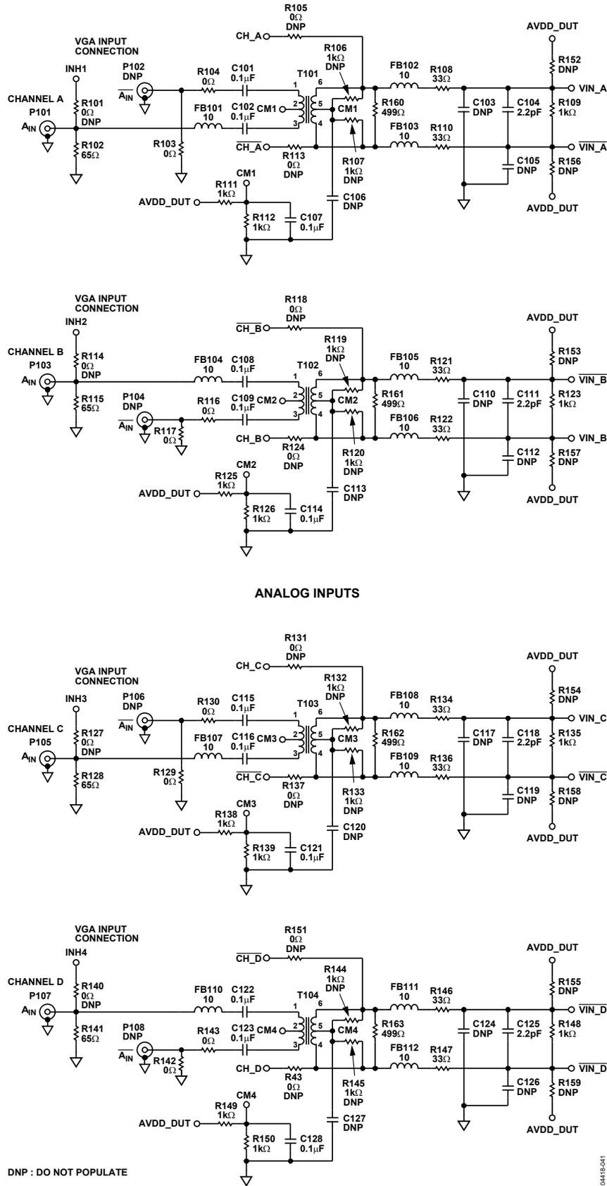
Figure 48. Evaluation Board Schematic, DUT Analog Inputs
