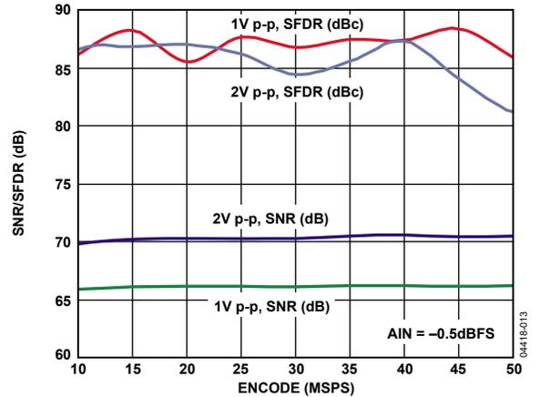
Figure 13. SNR/SFDR vs.  $f_{SAMPLE}$ ,  $f_{IN} = 10.3$  MHz,  $f_{SAMPLE} = 50$  MSPS
