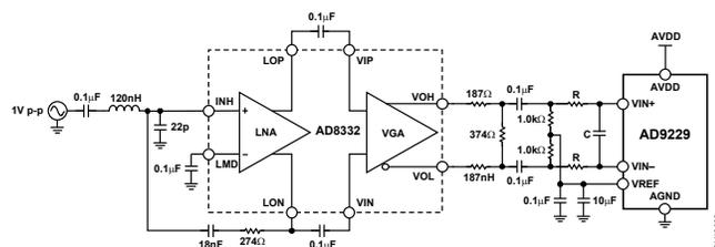
Figure 37. Differential Input Configuration Using the AD8332
