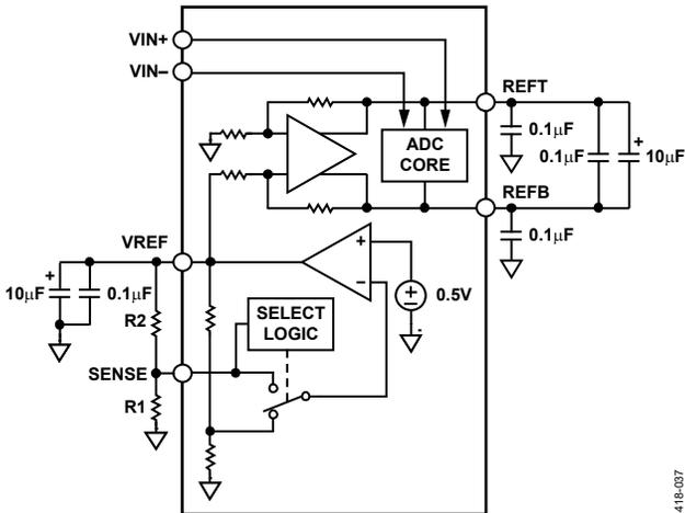
Figure 43. Programmable Reference Configuration
