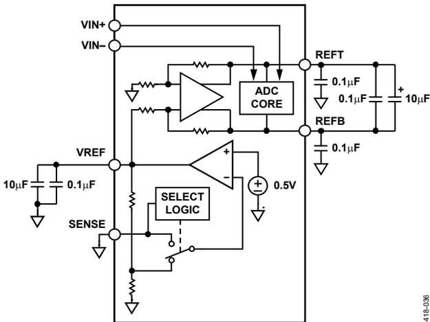
Figure 42. Internal Reference Configuration
