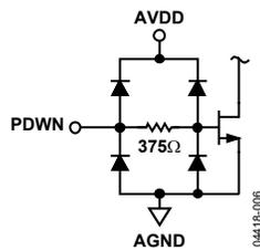
Figure 6. Equivalent Digital Input Circuit
