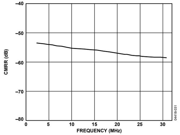
Figure 30. CMRR vs. Frequency,  $f_{\text{SAMPLE}} = 65 \text{ MSPS}$
