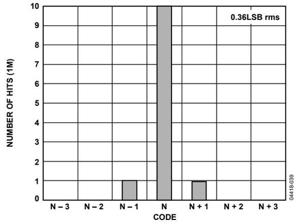
Figure 31. Input Referred Noise Histogram,  $f_{\text{SAMPLE}} = 65 \text{ MSPS}$
