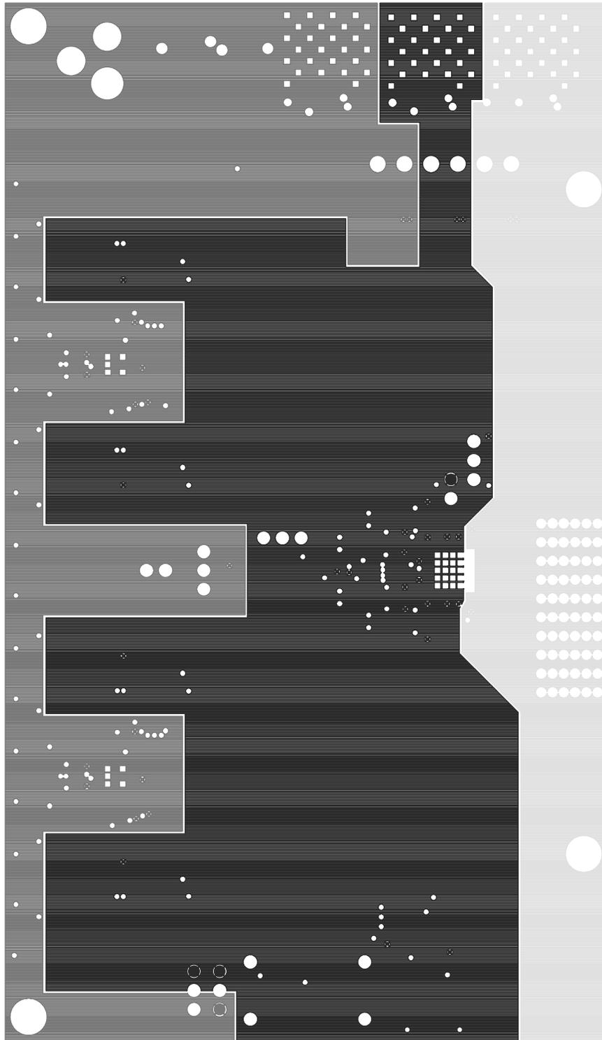
Figure 56. Evaluation Board Layout, Power Plane
