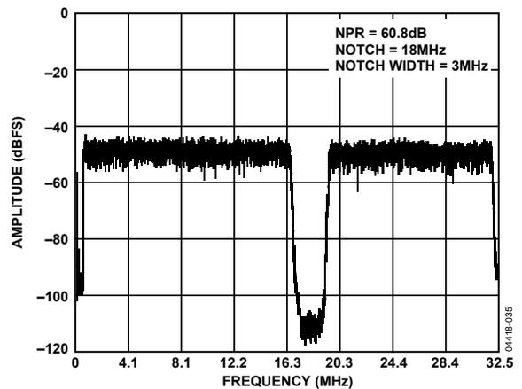
Figure 32. Noise Power Ratio (NPR),  $f_{\text{SAMPLE}} = 65 \text{ MSPS}$
