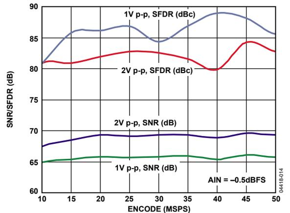
Figure 14. SNR/SFDR vs.  $f_{SAMPLE}$ ,  $f_{IN} = 25$  MHz,  $f_{SAMPLE} = 50$  MSPS
