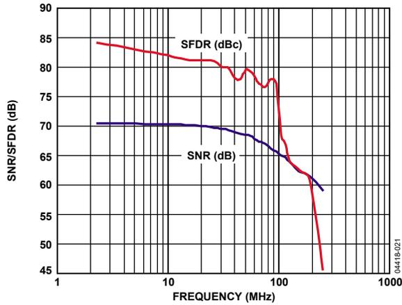
Figure 21. SNR/SFDR vs.  $f_{IN}$ ,  $f_{SAMPLE} = 65$  MHz
