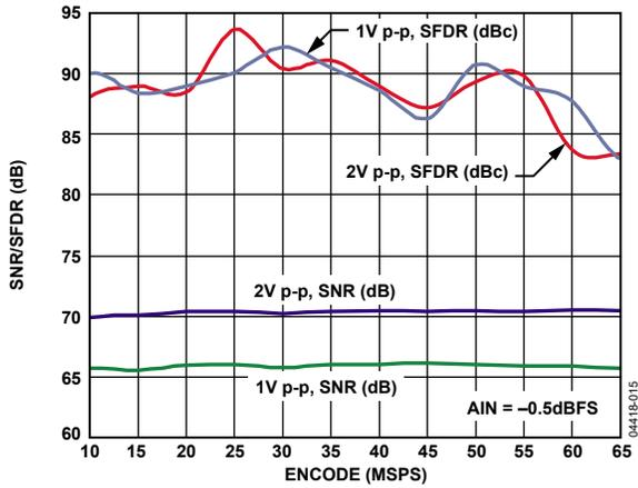
Figure 15. SNR/SFDR vs.  $f_{SAMPLE}$ ,  $f_{IN} = 10.3$  MHz,  $f_{SAMPLE} = 65$  MSPS
