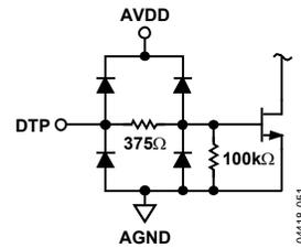
Figure 8. Equivalent DTP Input Circuit
