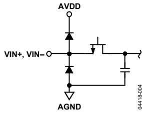
Figure 4. Equivalent Analog Input Circuit
