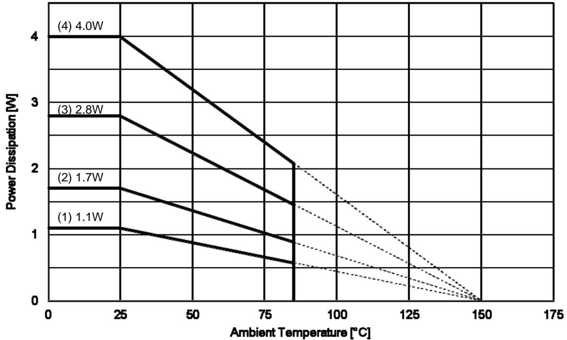
Figure 8. Power Dissipation
