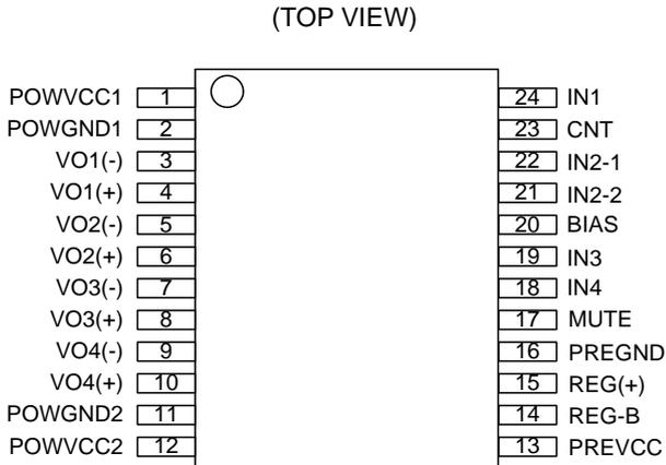
Figure 2. Pin Configuration
