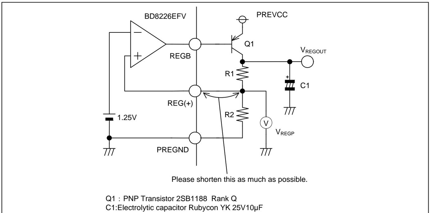
Figure 4. Regulator Block Diagram
