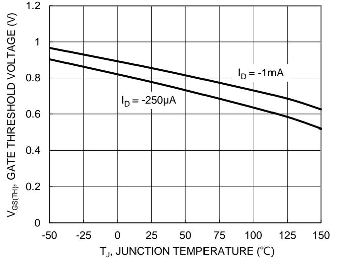
Figure 21. Gate Threshold Variation vs. Junction Temperature
