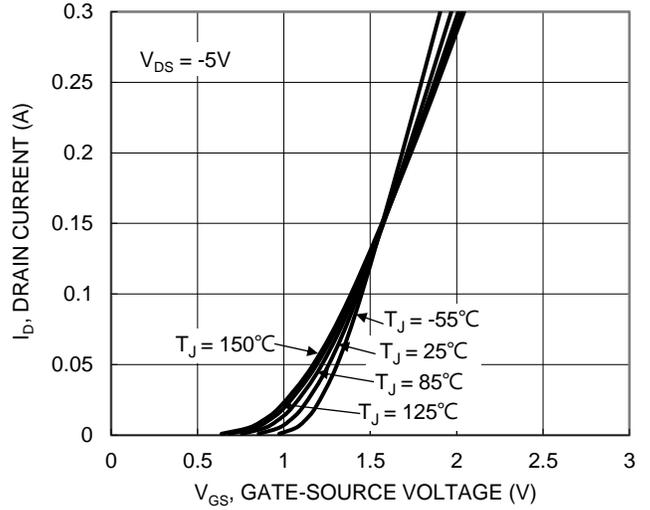
Figure 15. Typical Transfer Characteristic
