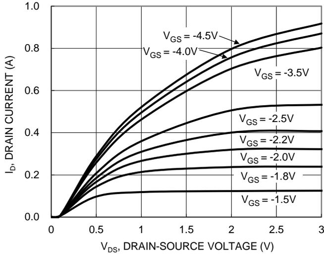
Figure 14. Typical Output Characteristic
