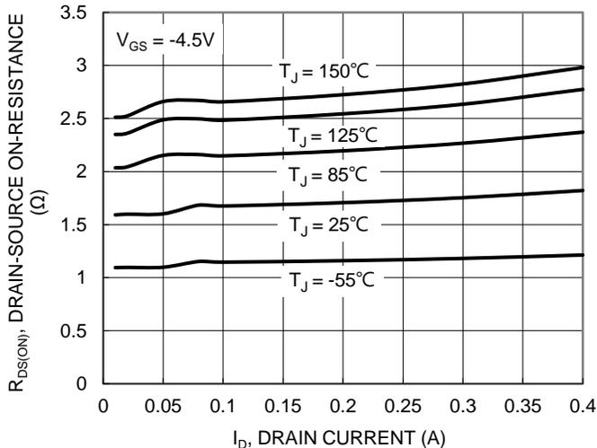
Figure 18. Typical On-Resistance vs. Drain Current and Junction Temperature
