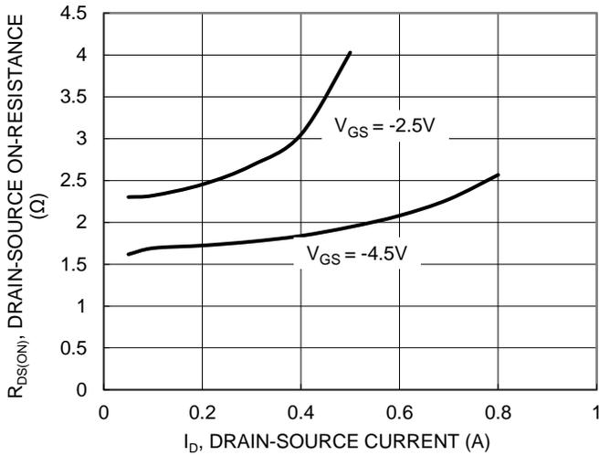
Figure 16. Typical On-Resistance vs. Drain Current and Gate Voltage
