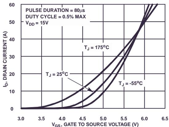
**Figure 7. Transfer Characteristics**
