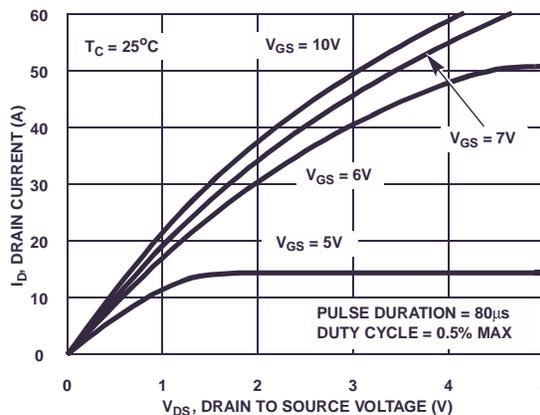
**Figure 8. Saturation Characteristics**
