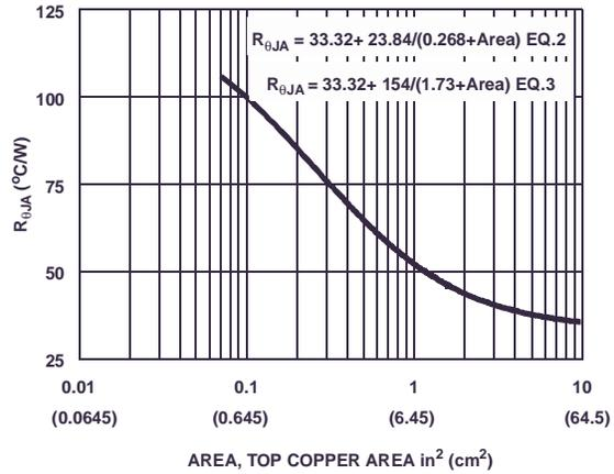
Figure 21. Thermal Resistance vs Mounting Pad Area
