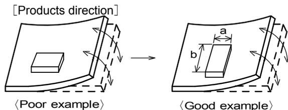
Products shall be located in the sideways direction (Length:a<b) to the mechanical stress.
