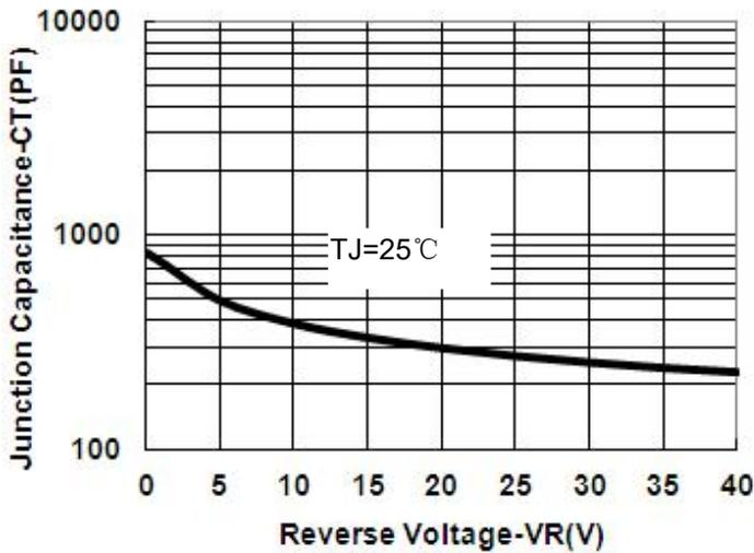
**Fig.1-Typical Junction Capacitance**
