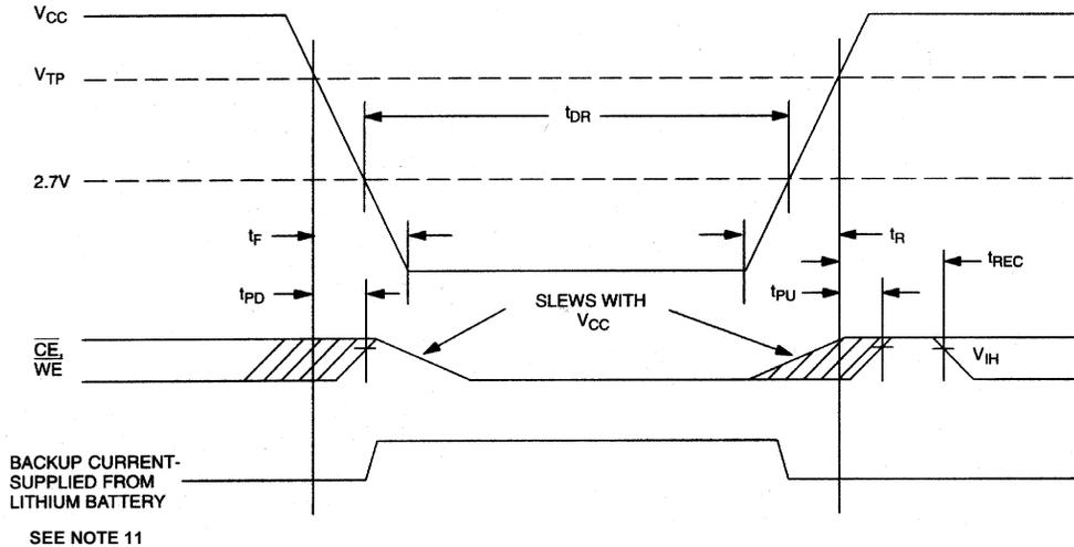
**POWER-DOWN/POWER-UP TIMING**(T<sub>A</sub>: See Note 10)
