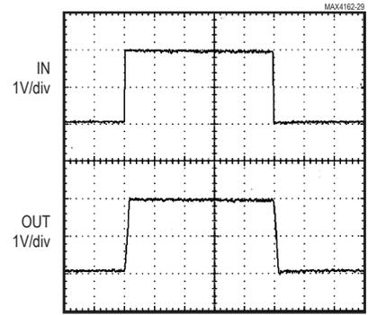
$V_{DD} = 3V$ ,  $V_{IN} = 2V$ ,  $R_L = 100k\Omega$  to  $V_{DD}/2$ ,
