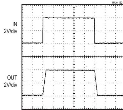
$V_{DD} = 5V$ ,  $V_{IN} = 4V$ ,  $R_L = 100k\Omega$  to  $V_{DD}/2$ ,
