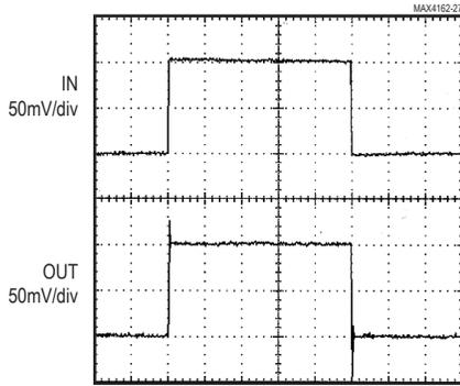
$V_{DD} = 5V$ ,  $V_{IN} = 100mV$ ,  $R_L = 100k\Omega$  to  $V_{DD}/2$ ,
