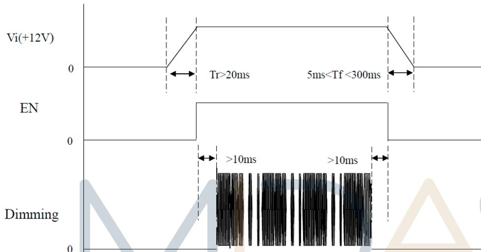
Note : While system is turned ON or OFF, the power sequences must follow as below descriptions Turn ON sequence:  $V_i(+12V) \rightarrow EN \rightarrow$  Dimming
