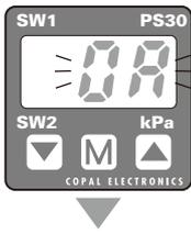
Release the applied pressure in the pressure port (i.e., let the pressure port be opened to the atmosphere).
