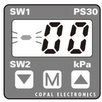
Press the **SW2** and **M** buttons simultaneously in Operations Mode. After switched to Initial Setting Mode, the third digit will blink. (The values **-00** for the 102R model and **-10** for the 103R have been set in the factory.)
