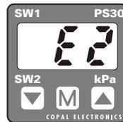
If pressure is applied during zero point adjustment, will be displayed.
