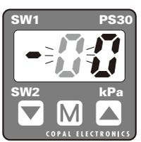
Press the **M** button to move to the next digit. The value of the digit may be set when the LED below the digit blinks. The number will change every time the **SW2** or **SW1** button is pressed.
