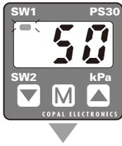
Press the **M** and **▲** buttons simultaneously in Operations Mode.
