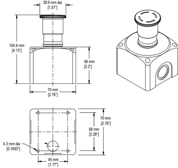
Figure 3. SSA-EBM-xxL E-Stop Buttons
