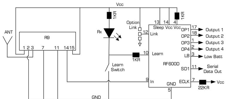
The Receiver application circuits generates a receiver decoder with four relay drive outputs and serial data output. It has easy Learn feature of the Keeloq transmitter and provides a Transmitter lower Battery indication.
