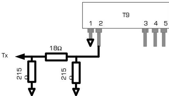
When laying out this network, keep all tracks as short as possible, especially ground paths and use 50 ohm track impedances when connecting to and from this network. This impedance can be realised on 1.6mm FR4 pcb by using a track width of 2.5mm.
