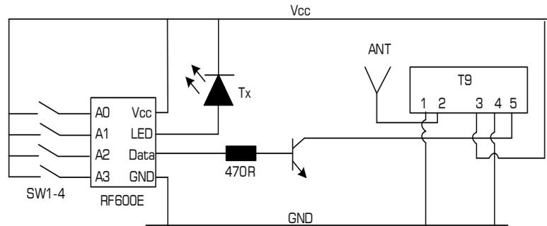
The transmitter application circuits generates a highly secure Keeloq protocol four switch transmitter encoder with LED indication or Transmission.
