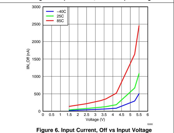
Figure 6. Input Current, Off vs Input Voltage
