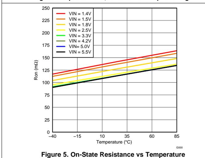
Figure 5. On-State Resistance vs Temperature
