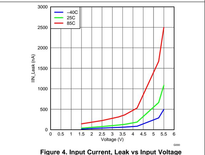
Figure 4. Input Current, Leak vs Input Voltage
