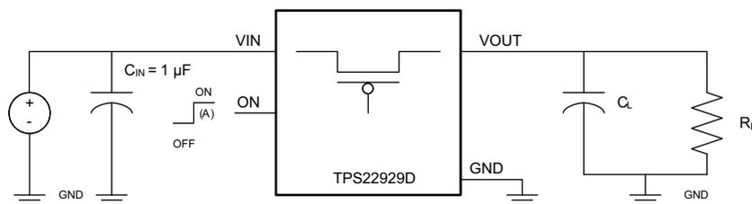
A. Rise and fall times of the control signal is 100 ns.
