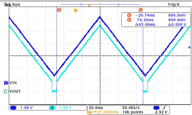
Figure 8. Under-Voltage Lockout Response (IOUT = -100mA)
