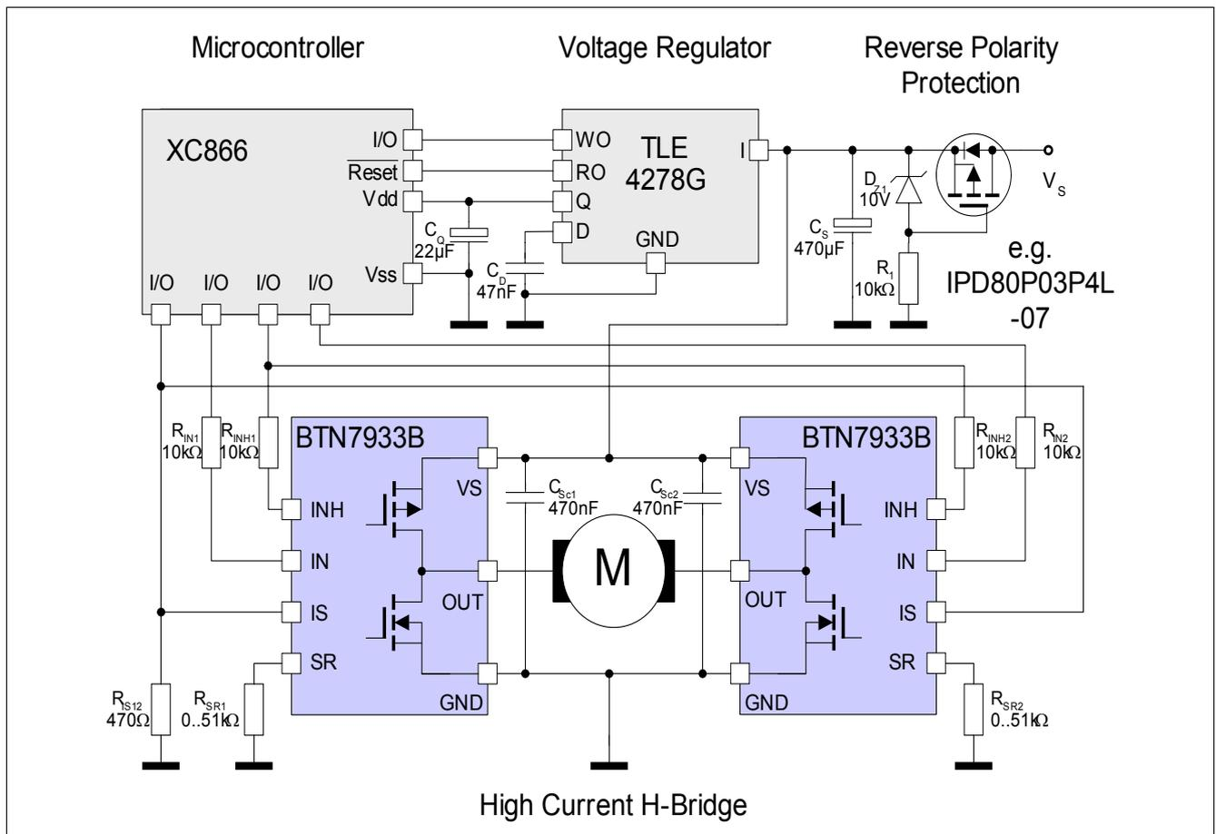
Figure 14 Application Example: H-Bridge with two BTN7933B
