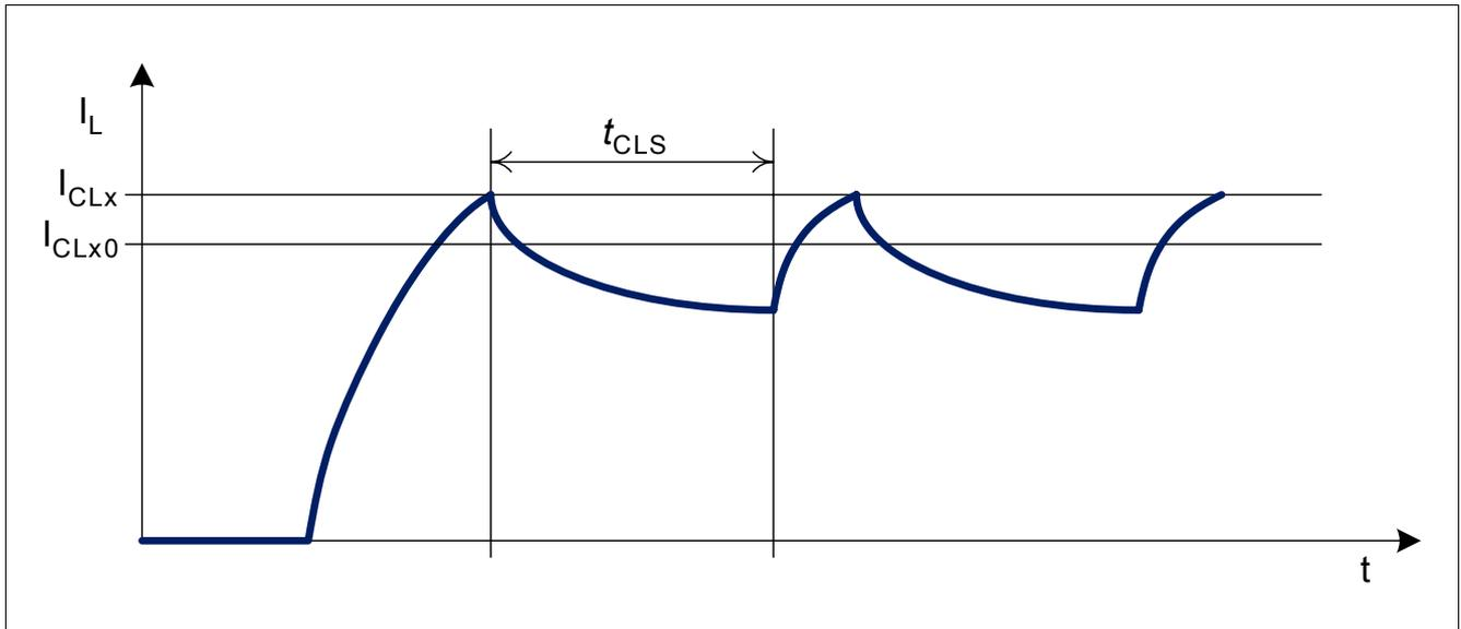
Figure 9 Timing Diagram Current Limitation (Inductive Load)
