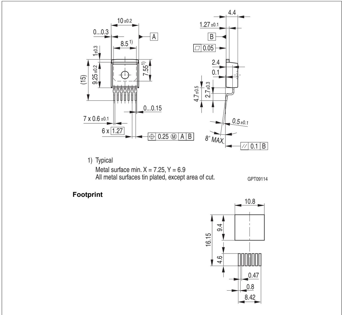
Figure 16 PG-TO263-7-1 (Plastic Green Transistor Single Outline Package)
