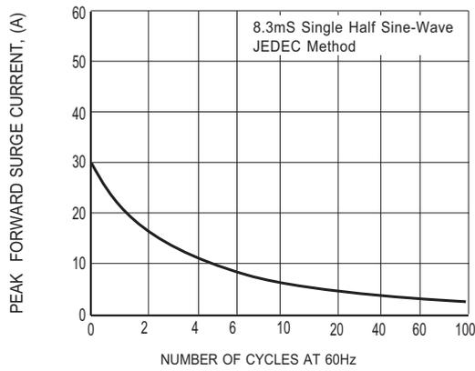
FIG. 1 - MAXIMUM NON-REPETITIVE FORWARD SURGE CURRENT
