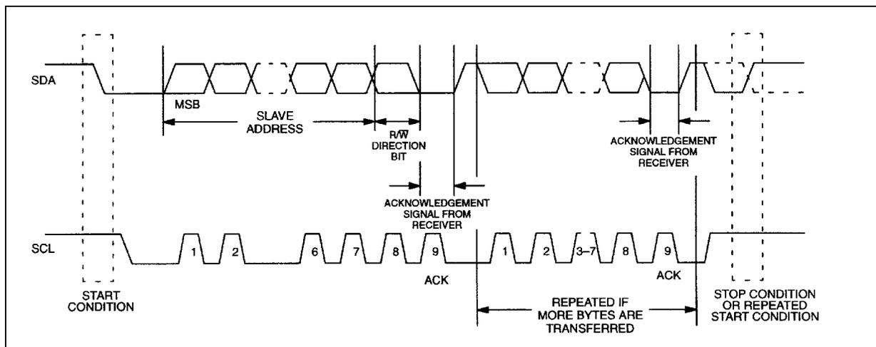
Figures 2, 3, and 4 detail how data transfer is accomplished on the 2-wire bus. Depending upon the state of the R/W bit, two types of data transfer are possible:
