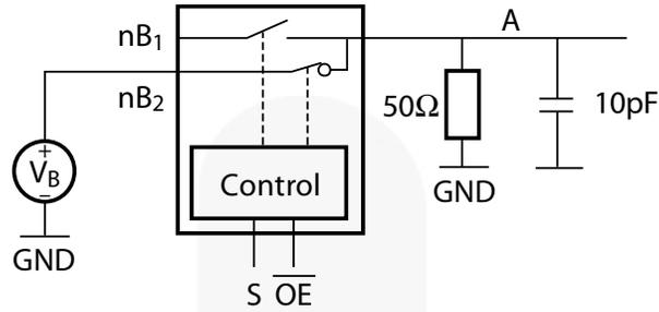
Notes: Input driven by 50Ω source terminated in 50Ω.
