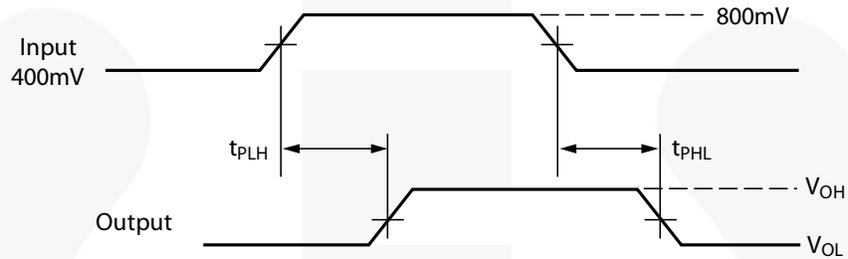
Figure 14. Propagation Delay
