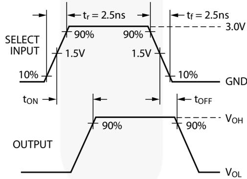
**Figure 10. AC Waveforms**
