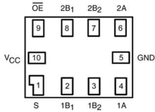
Figure 1. MicroPak™ (Top View)
