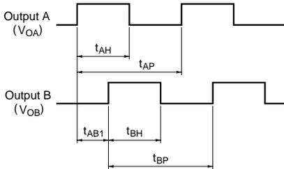
Rotational direction: Counterclockwise when seen from OPIIC light detector
