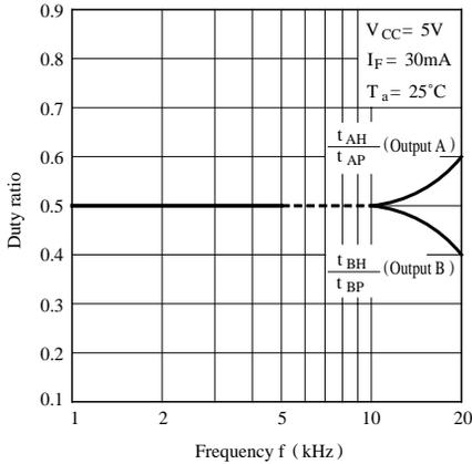
Fig. 4 Phase Difference vs. Frequency
