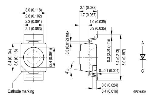
Approximate Weight:34.0 mgPackage marking:CathodeCorrosion test:Class: 3B
