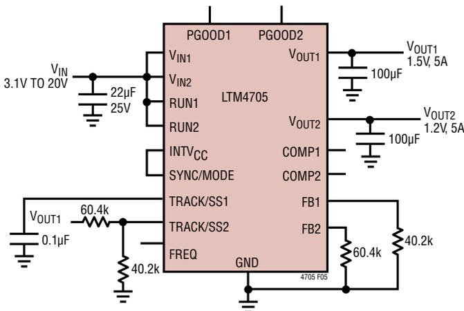
Figure 5. Example Schematic of Ratiometric Output Voltage Tracking
