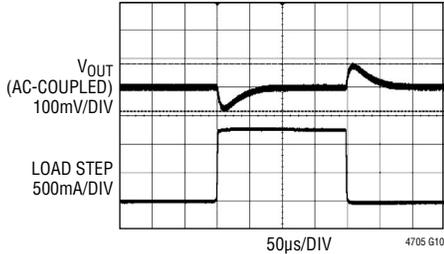
$V_{IN} = 12V$ ,  $V_{OUT} = 5V$ ,  $f_{SW} = 1MHz$
