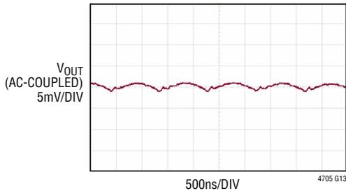
$V_{IN} = 12V$ ,  $V_{OUT} = 1V$ ,  $f_{SW} = 1MHz$
