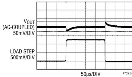
V<sub>IN</sub> = 12V, V<sub>OUT</sub> = 1.2V, f<sub>SW</sub> = 1MHz
