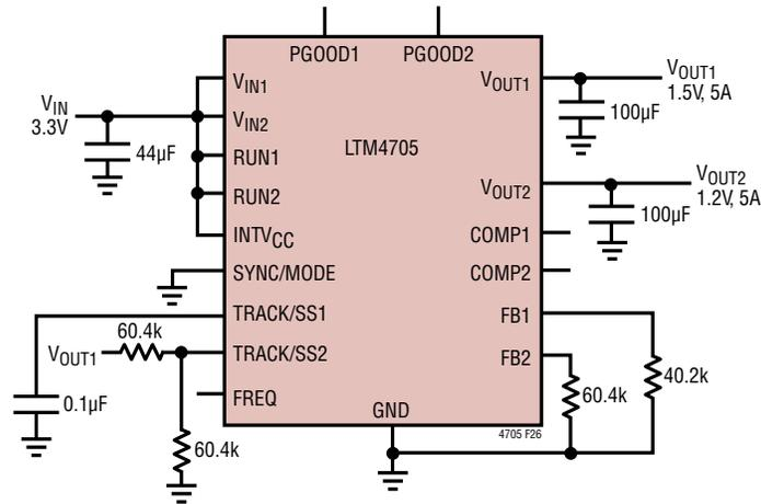
Figure 26. 3.3V<sub>IN</sub>, 1.5V and 1.2V Output at 5A Design with Output Coincident Tracking
