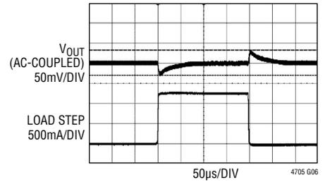
V<sub>IN</sub> = 12V, V<sub>OUT</sub> = 1.5V, f<sub>SW</sub> = 1MHz
