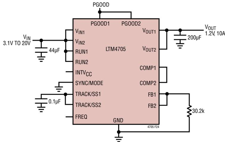
Figure 24. 3.1V<sub>IN</sub> to 20V<sub>IN</sub>, 1.2V Two Phase in Parallel 10A Design
