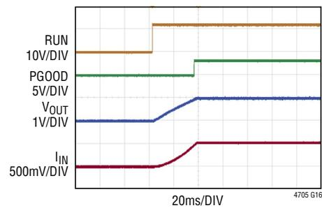
$V_{IN} = 12V$ ,  $V_{OUT} = 1V$ ,  $f_{SW} = 1MHz$ ,
