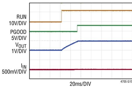
$V_{IN} = 12V$ ,  $V_{OUT} = 1V$ ,  $f_{SW} = 1MHz$ ,
