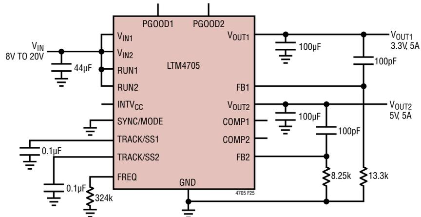
Figure 25. 8V<sub>IN</sub> to 20V<sub>IN</sub>, 3.3V and 5V Output at 5A with 2MHz Switching Frequency
