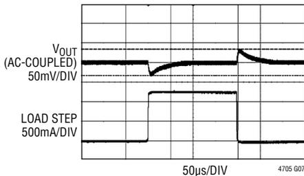
V<sub>IN</sub> = 12V, V<sub>OUT</sub> = 1.8V, f<sub>SW</sub> = 1MHz
