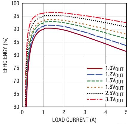
**Efficiency vs Load Current from 12V<sub>IN</sub>**
