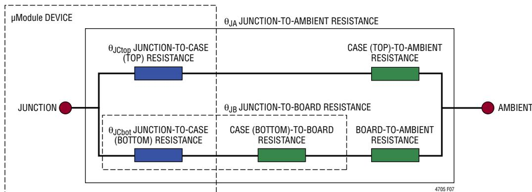
Figure 7. Graphical Representation of JESD51-12 Thermal Coefficients
