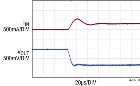
$V_{IN} = 12V$ ,  $V_{OUT} = 1.0V$ ,  $f_{SW} = 1MHz$
