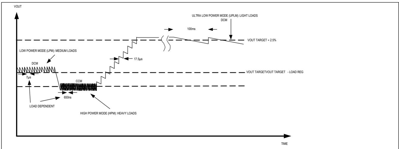
Figure 5. ULPM, LPM, and HPM Waveforms (Part 2)
