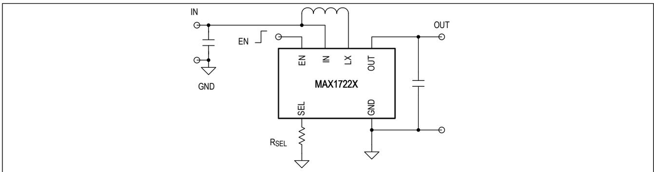
Figure 6. Single  $R_{SEL}$  Resistor Sets the Output Voltage
