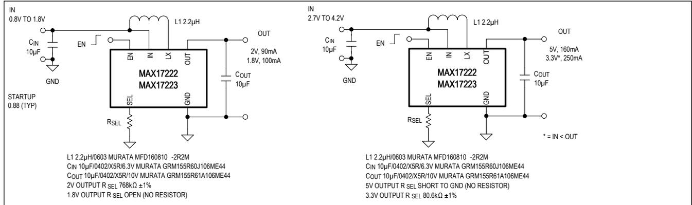
Highest Efficiency Solution—4mm x 4mm Inductor—MAX17222/MAX17223 500mA I<sub>LIM</sub> (Part 1)
