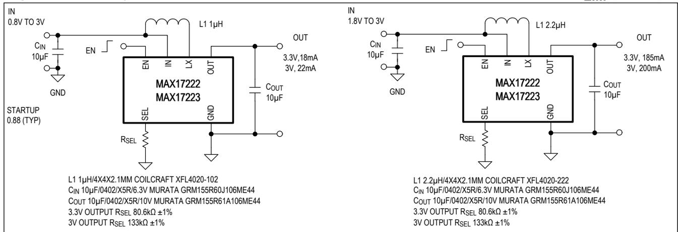
Highest Efficiency Solution—4mm x 4mm Inductor—MAX17222/MAX17223 500mA I<sub>LIM</sub> (Part 2)
