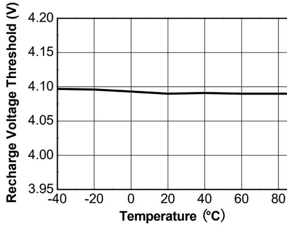
Figure 22. Recharge Voltage Threshold vs Temperature
