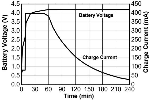
Figure 4. Complete Charge Cycle
