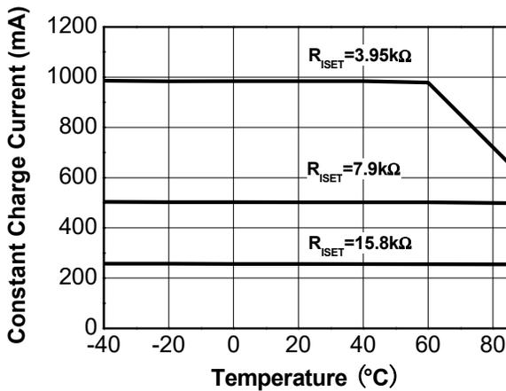
Figure 18. Constant Charge Current vs Temperature
