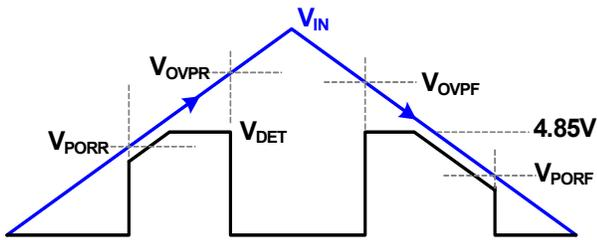
Figure 28. DET Pin Output Voltage vs Input Voltage
