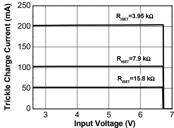
Figure 9. Trickle Charge Current vs  $V_{IN}$
