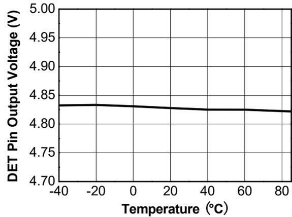
Figure 25. DET Pin Output Voltage vs Temperature
