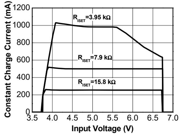
Figure 8. Constant Charge Current vs  $V_{IN}$
