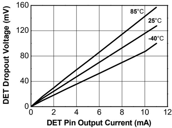
Figure 16. DET Dropout Voltage vs Output Current
