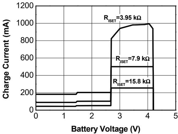
Figure 10. Charge Current vs Battery Voltage
