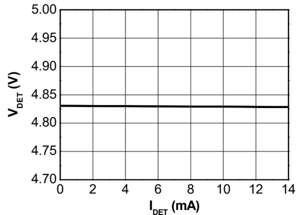
Figure 15. DET Pin Output Voltage vs Output Current
