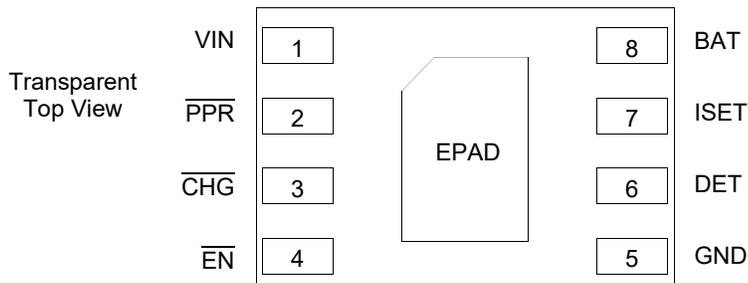
Figure 3. 34675 Pin Connections
