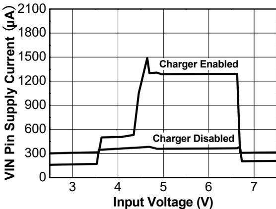
Figure 6. VIN Pin Supply Current vs  $V_{IN}$
