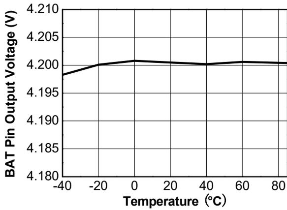
Figure 17. Charger Output Voltage vs Temperature
