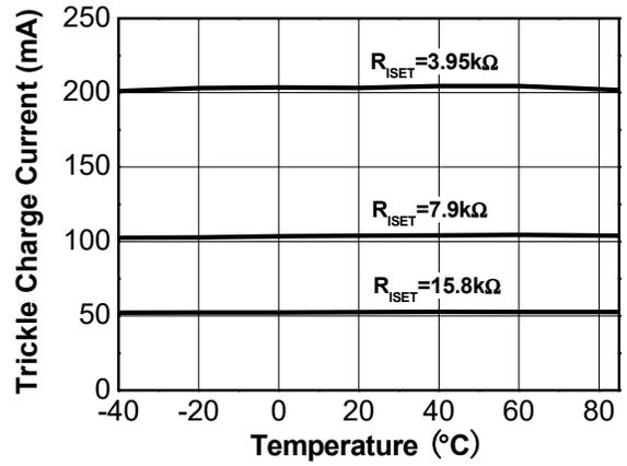
Figure 19. Trickle Charge Current vs Temperature
