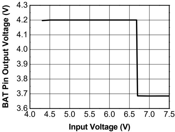
Figure 5. Charger Output Voltage vs  $V_{IN}$
