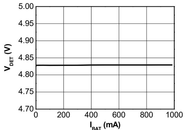
Figure 14. DET Pin Output Voltage vs Charge Current
