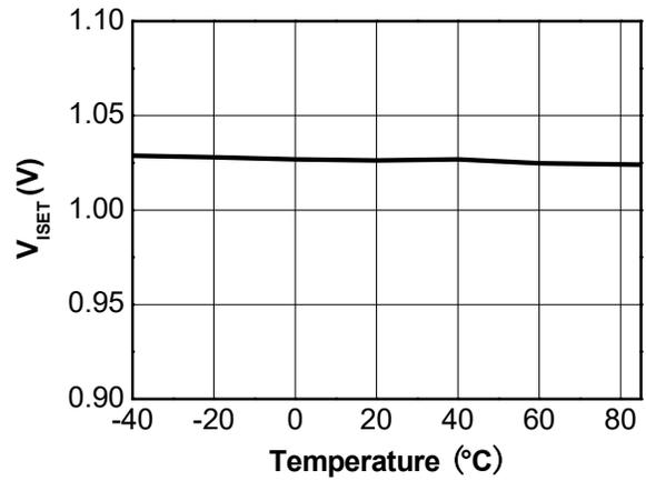
Figure 20.  $V_{ISET}$  vs Temperature
