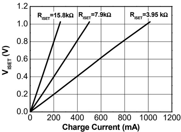
Figure 12.  $V_{ISET}$  vs Charge Current
