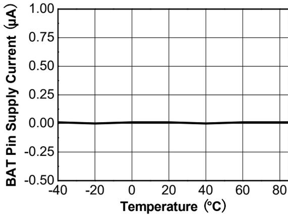
Figure 23. BAT Pin Supply Current vs Temperature
