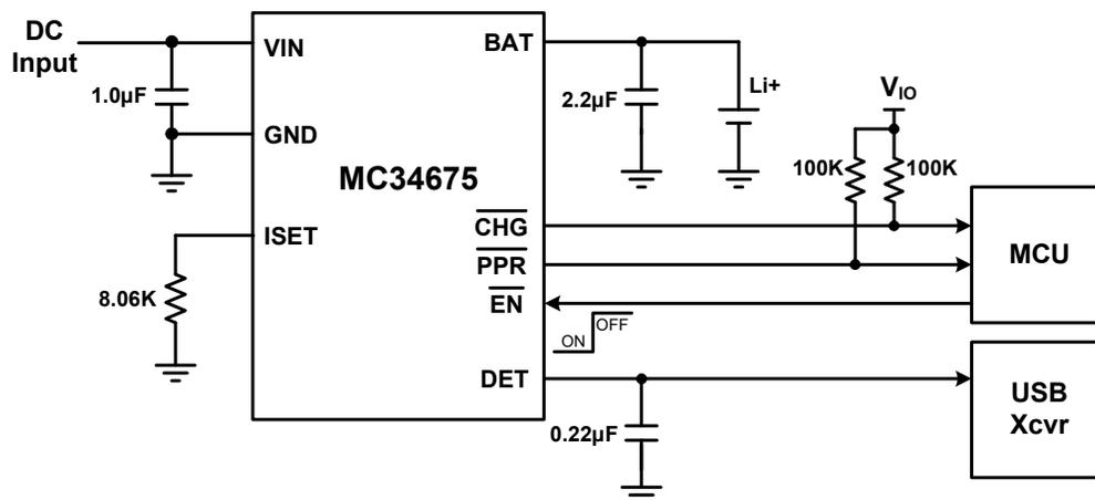
Figure 30. Li+ Battery Charger in Handheld System
