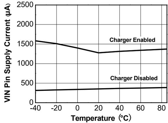
Figure 24. VIN Pin Supply Current vs Temperature
