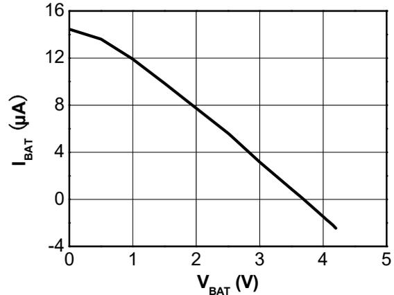
Figure 7. BAT Pin Current vs Battery Voltage in OVP
