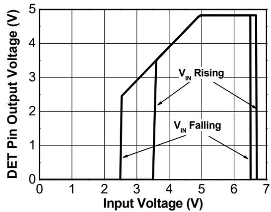
Figure 13. DET Pin Output Voltage vs Input Voltage
