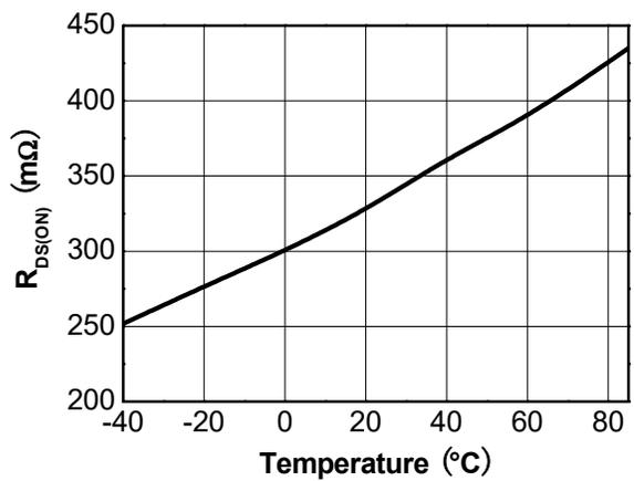
Figure 21.  $R_{DS(ON)}$  vs Temperature
