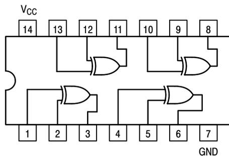
Figure 1. Pinout: 14-Lead Packages Conductors
