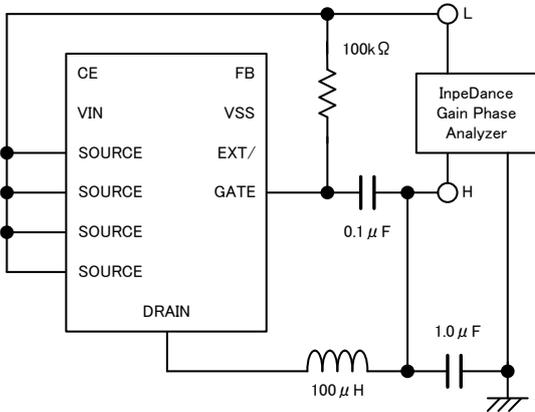
Input Capacitance:  $C_{iss} = C_{gd} + C_{gs}$
