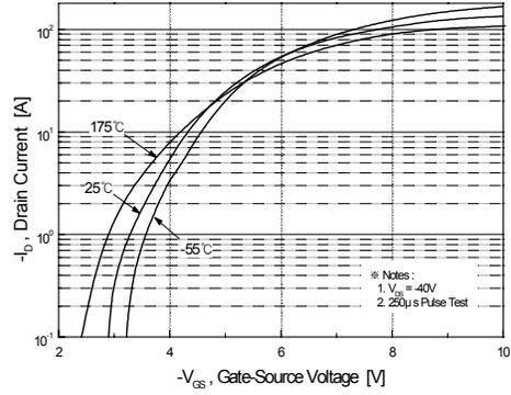
Figure 2. Transfer Characteristics
