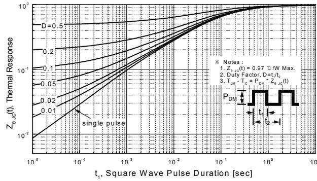
**Figure 11. Transient Thermal Response Curve**
