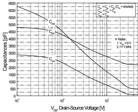
Figure 5. Capacitance Characteristics
