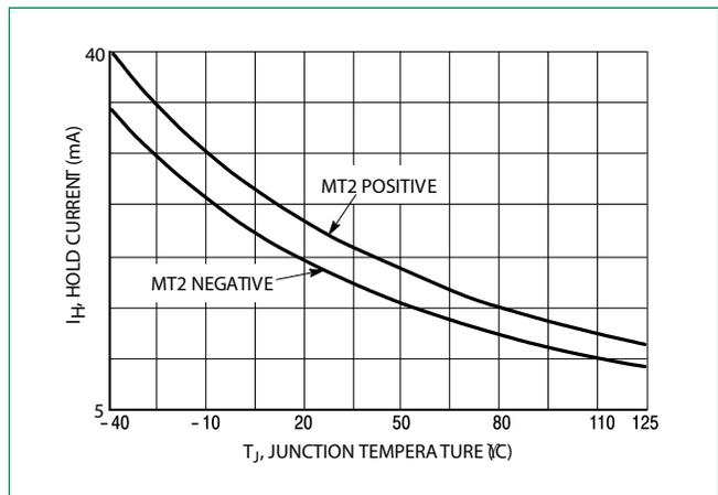
**Figure 6. Typical Holding Current vs Junction Temperature**
