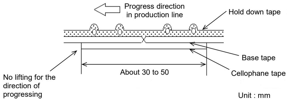
b) When hold down tape is spliced
