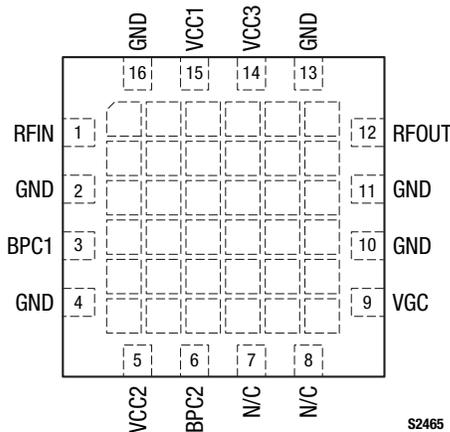
**Figure 2. SKY65375-11 Pinout – 16-Pin MCM (Top View)**
