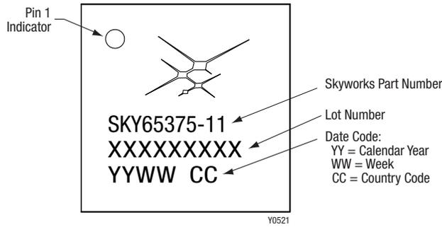
Figure 8. Typical Part Marking
