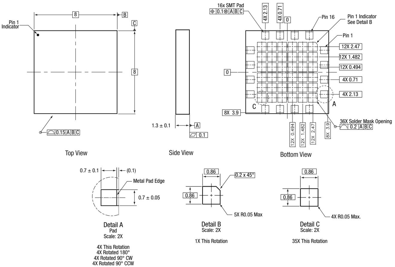
Dimensioning and tolerancing according to ASME Y14.5M-1994.
