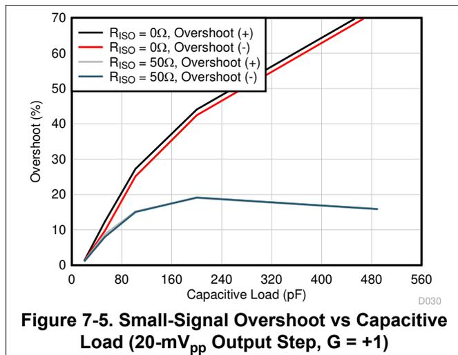
Figure 7-5. Small-Signal Overshoot vs Capacitive Load (20-mV<sub>pp</sub> Output Step, G = +1)
