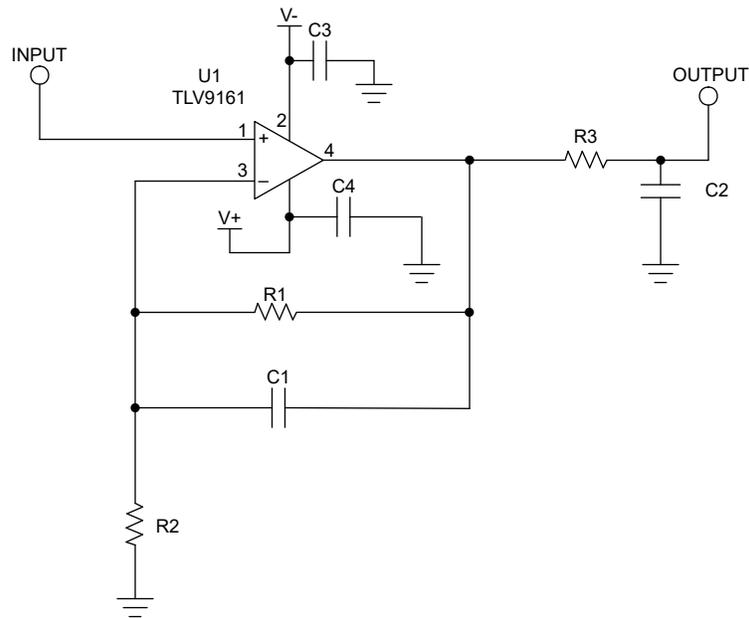
Figure 10-1. Schematic for Noninverting Configuration Layout Example
