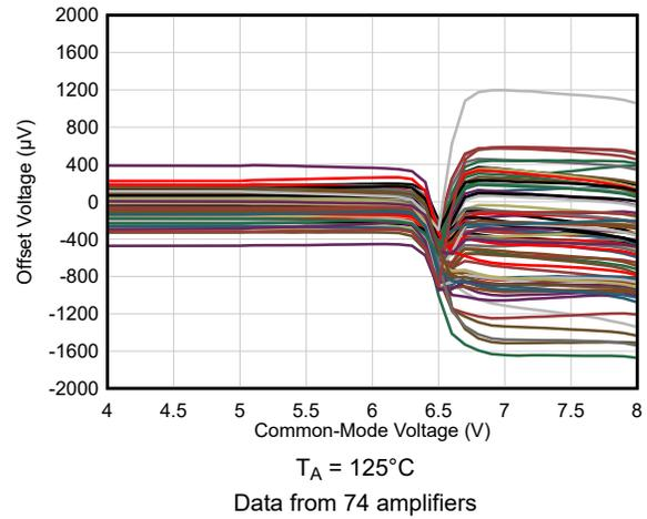
**Figure 6-8. Offset Voltage vs Common-Mode Voltage (Transition Region)**
