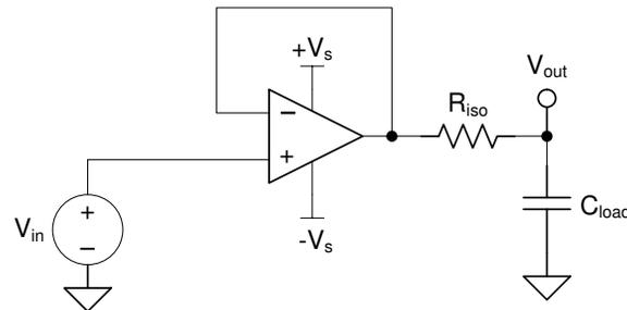
**Figure 7-7. Extending Capacitive Load Drive With the TLV9161**
