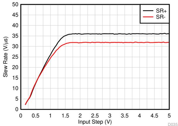
**Figure 6-15. Slew Rate vs Input Step Voltage**
