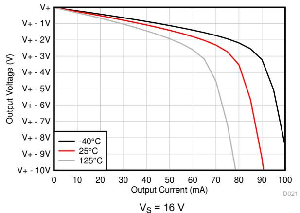
**Figure 6-16. Output Voltage Swing vs Output Current (Sourcing)**
