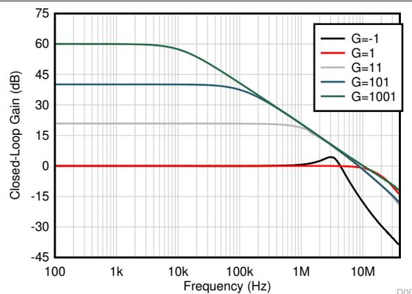
**Figure 6-12. Closed-Loop Gain vs Frequency**
