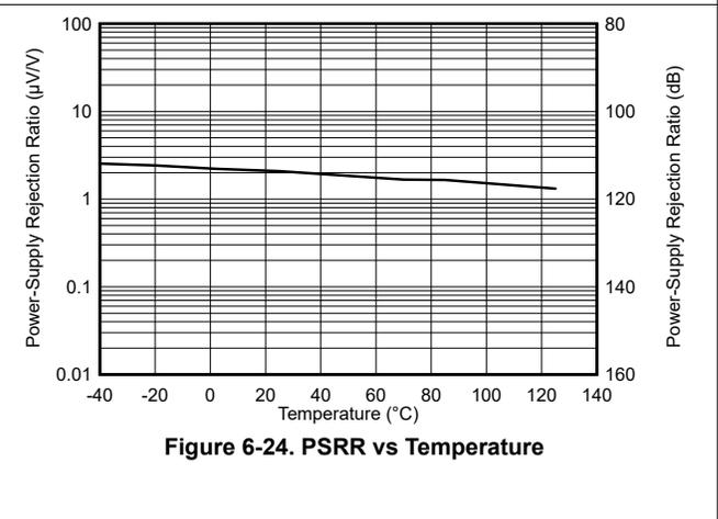
**Figure 6-24. PSRR vs Temperature**
