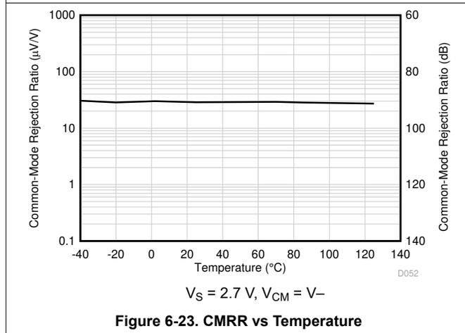
**Figure 6-23. CMRR vs Temperature**
