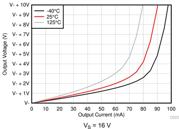
**Figure 6-17. Output Voltage Swing vs Output Current (Sinking)**
