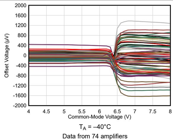
**Figure 6-10. Offset Voltage vs Common-Mode Voltage (Transition Region)**
