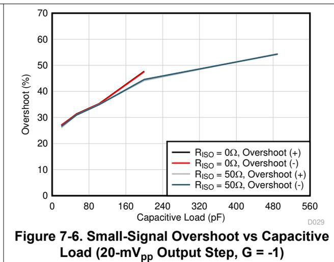
Figure 7-6. Small-Signal Overshoot vs Capacitive Load (20-mV<sub>pp</sub> Output Step, G = -1)
