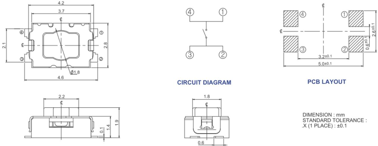
**Figure 2 – 223JMV...G, Surface Mount Gull Wing, Actuator Height 1.9mm, With Ground Terminal**
