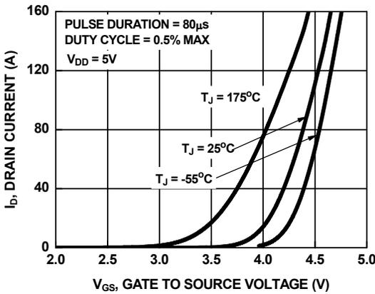
Figure 7. Transfer Characteristics
