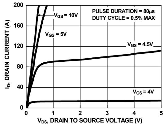
Figure 8. Saturation Characteristics
