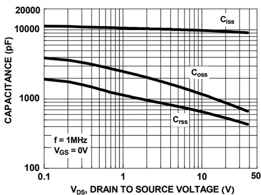
Figure 13. Capacitance vs Drain to Source Voltage
