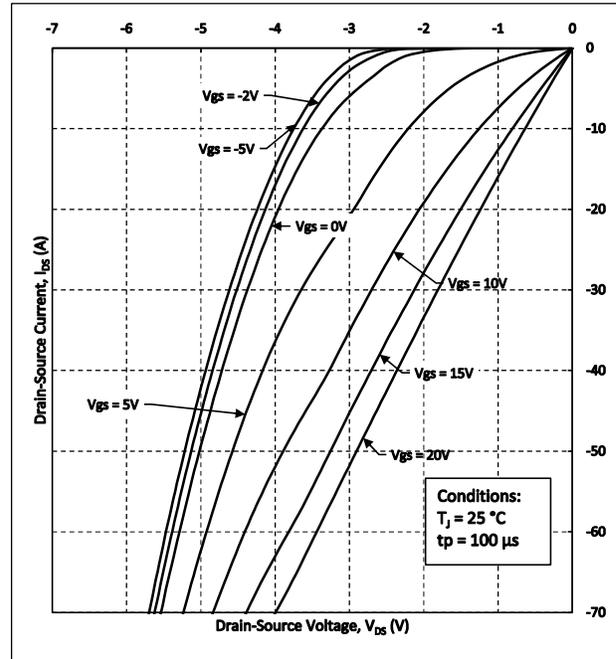
Figure 10. Body Diode Characteristics at  $T_J = 25^\circ\text{C}$
