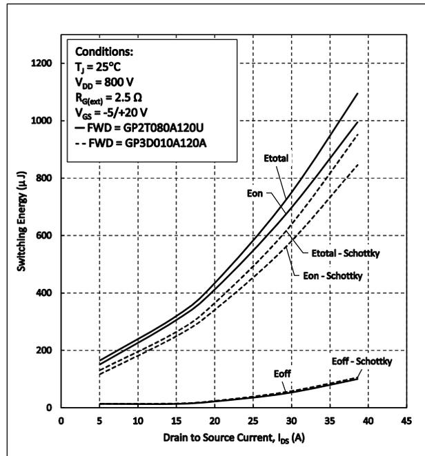
Figure 20. Clamped Inductive Switching Energy vs. Drain Current
