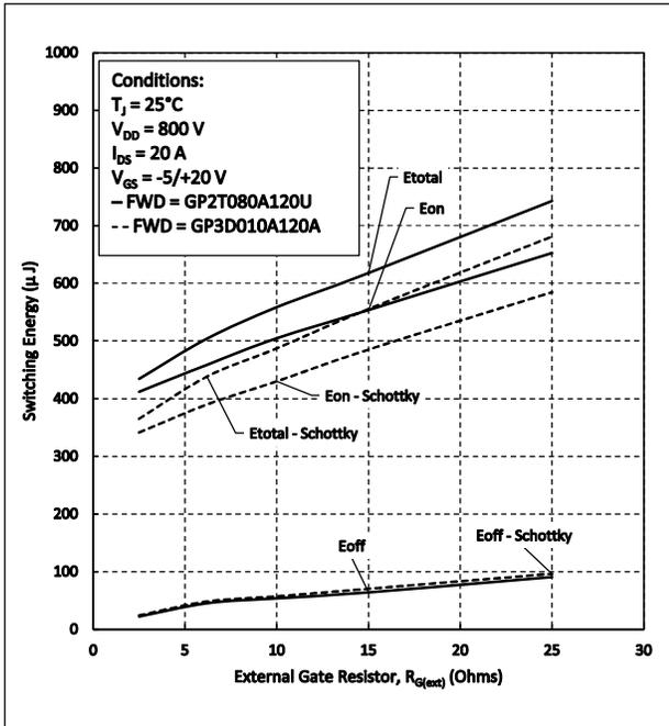
Figure 21. Clamped Inductive Switching Energy vs.  $R_{G(ext)}$
