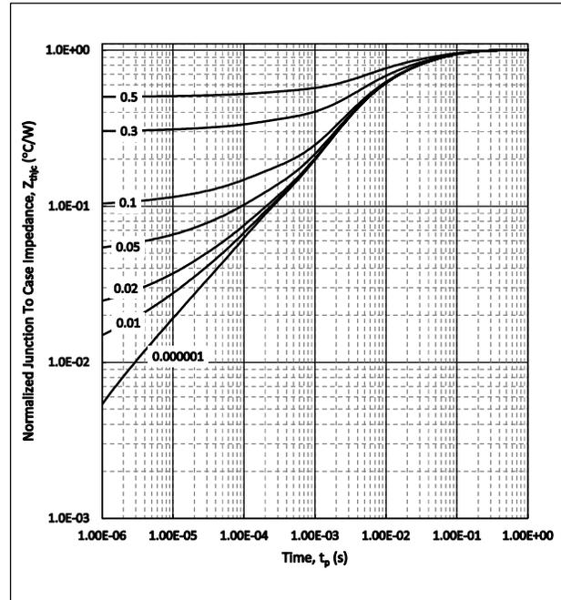
Figure 18. Transient Thermal impedance (Junction to Case)
