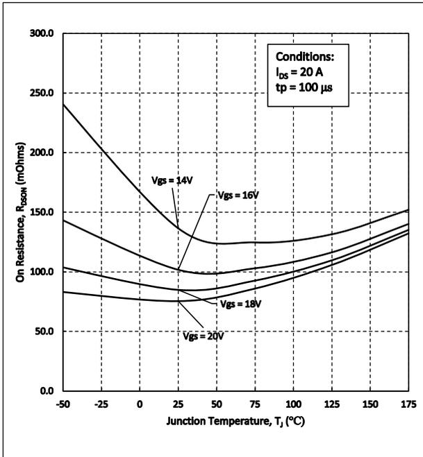
Figure 7. On-Resistance vs. Temperature For Various Gate Voltages
