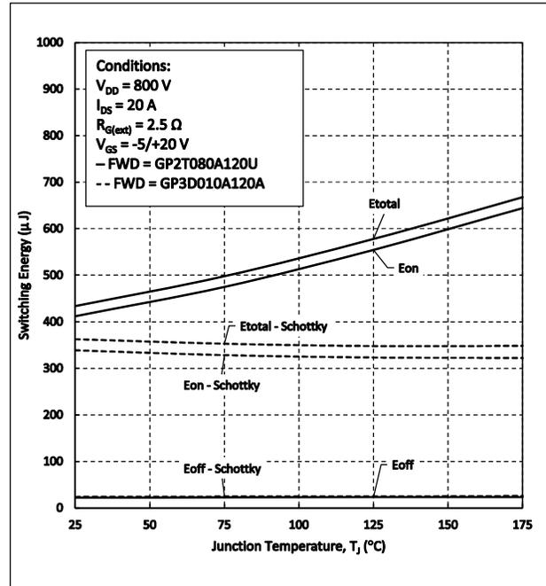
Figure 22. Clamped Inductive Switching Energy vs. Temperature
