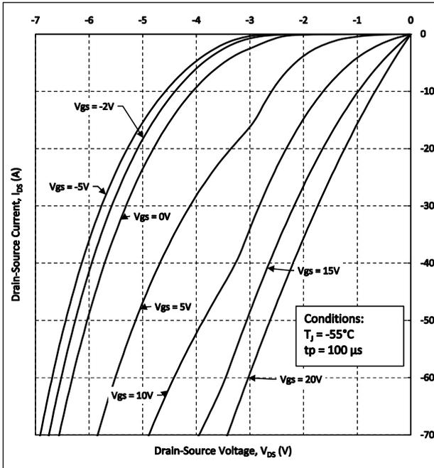
Figure 9. Body Diode Characteristics at  $T_J = -55^\circ\text{C}$
