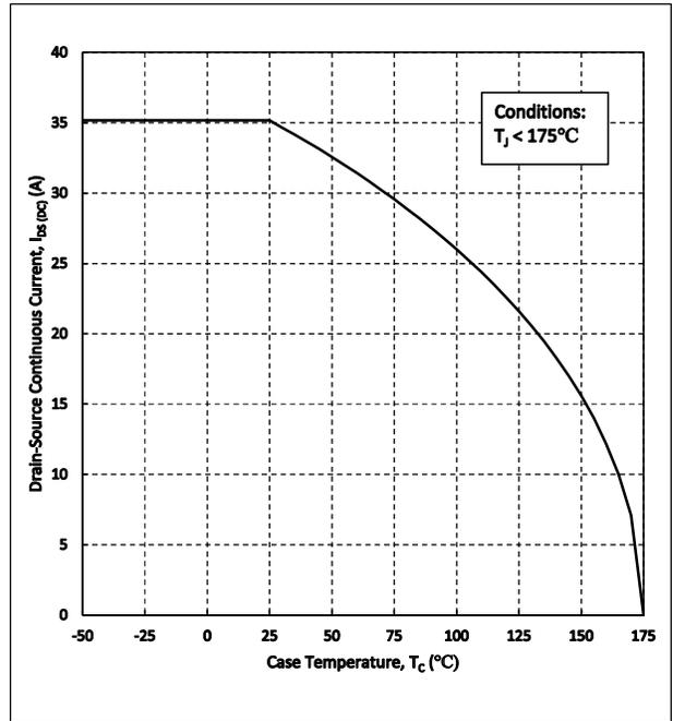
Figure 16. Continuous Drain Current Derating vs. Case Temperature
