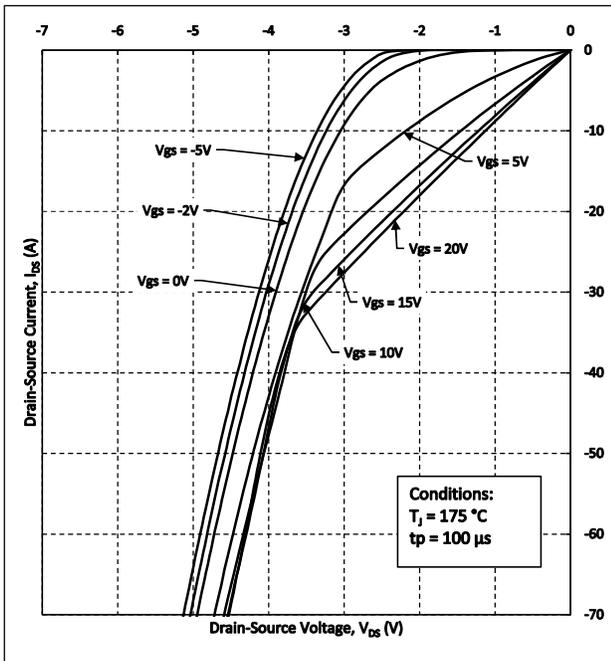
Figure 11. Body Diode Characteristics at  $T_J = 175^\circ\text{C}$
