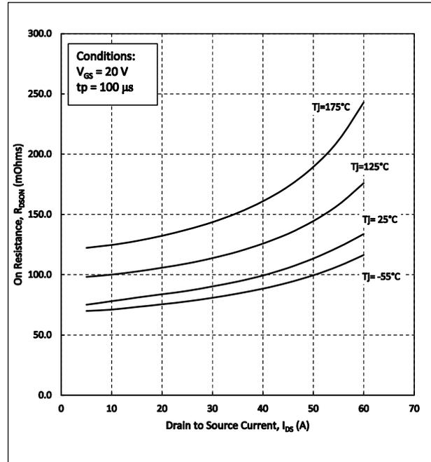
Figure 6. On-Resistance vs. Drain Current For Various Temperature
