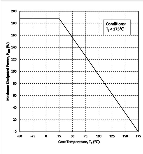
Figure 17. Maximum Power Dissipation Derating vs Case Temperature
