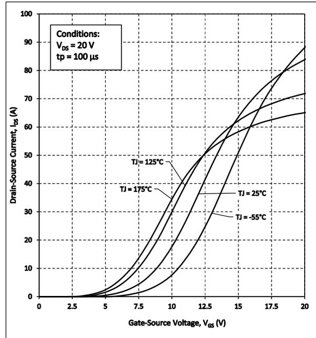
Figure 8. Transfer Characteristic for Various Junction Temperatures
