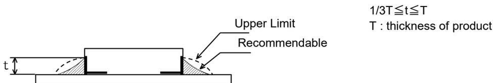
Accordingly increasing the solder volume, the mechanical stress to Chip is also increased. Exceeding solder volume may cause the failure of mechanical or electrical performance and become easy to tilt.
