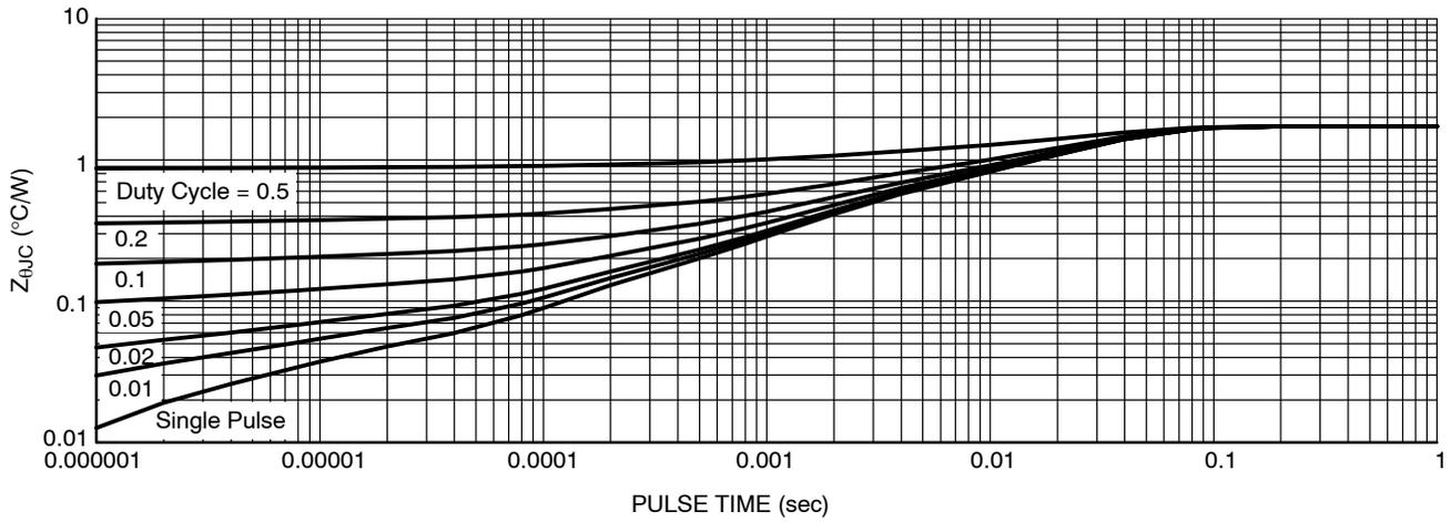
Figure 13. Thermal Impedance
